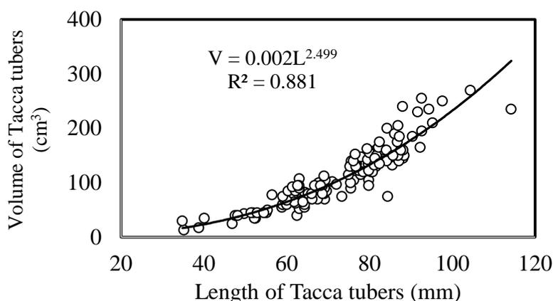
Figure 4: Volume model of Tacca tubers on length at average moisture content of 73.3% (wet basis)
