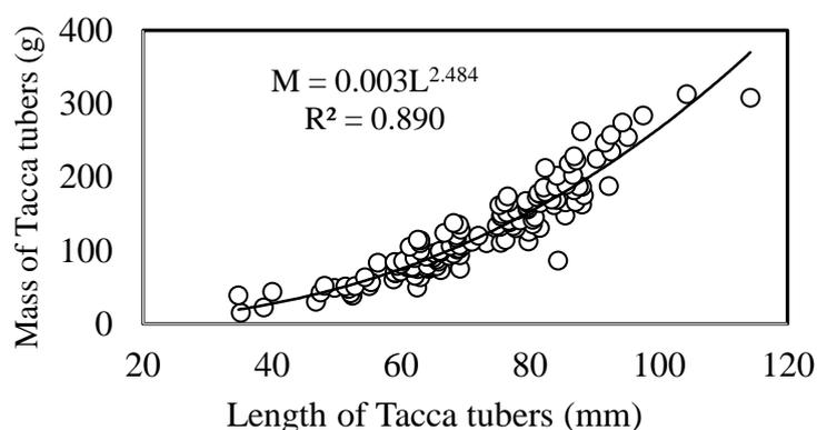
Figure 3: Mass model of Tacca tubers on length at average moisture content of 73.3% (wet basis)
