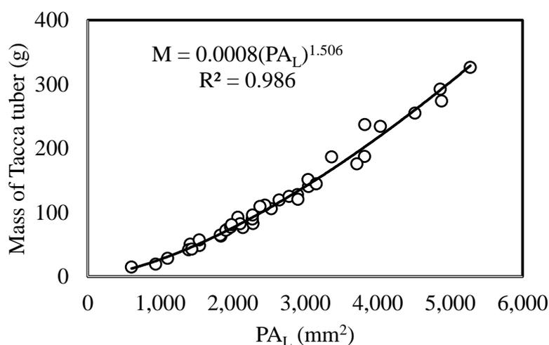
Figure 5: Mass model of Tacca tubers on  $PA_L$  at average moisture content of 73.3% (wet basis)
