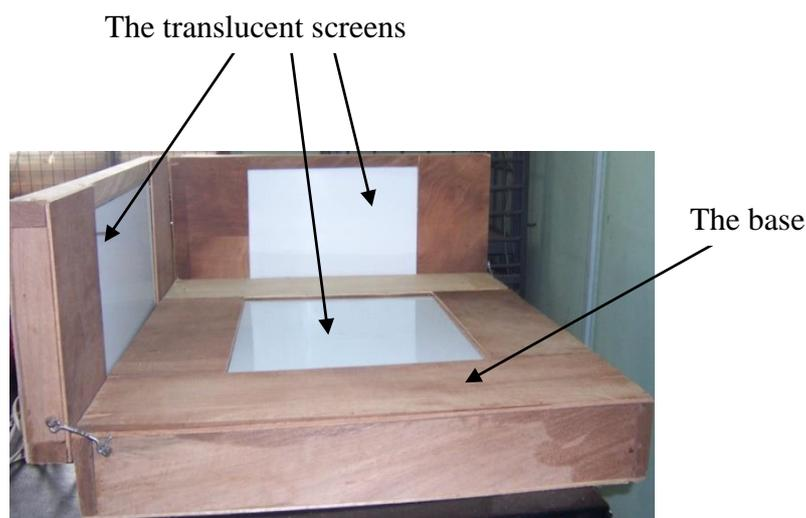
Figure 2: The image acquisition lighting box
