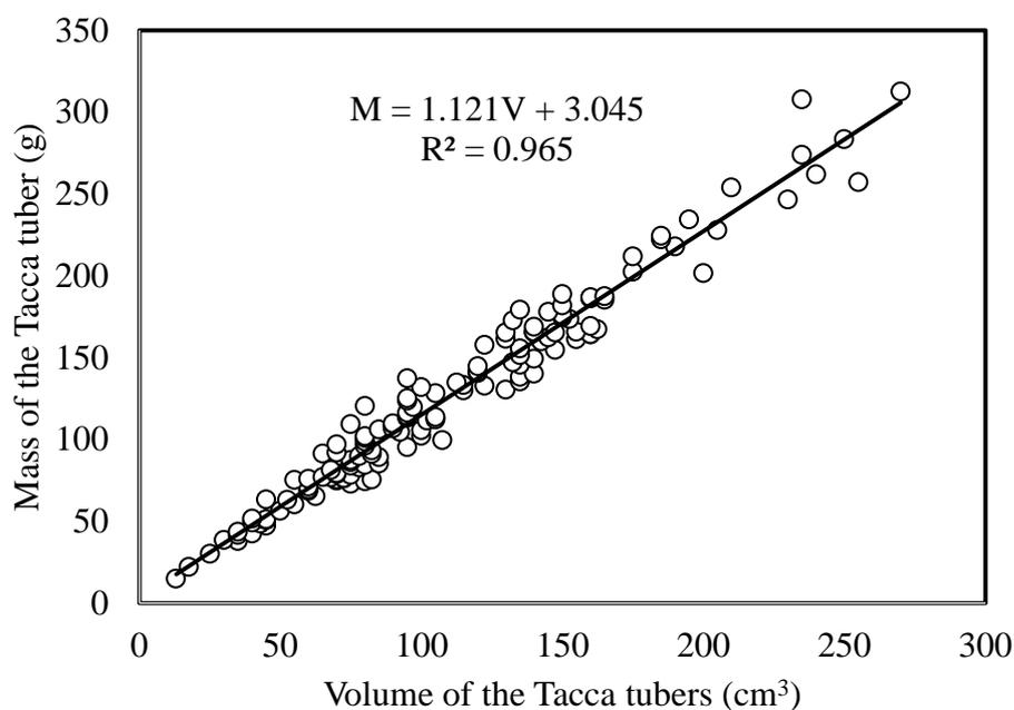
Figure 7: Mass model of Tacca tubers on volume at average moisture content of 73.3% (wet basis)
