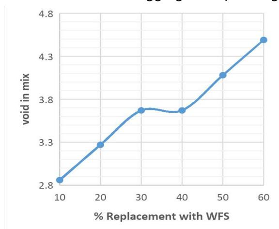
Figure 15: Void in mix (VIM) against different percentage replacement with WFS
