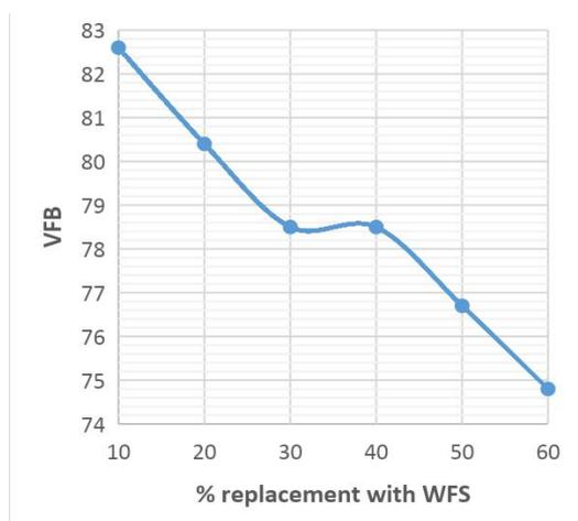
Figure 16: Void filled with bitumen against different percentage replacement with WFS
