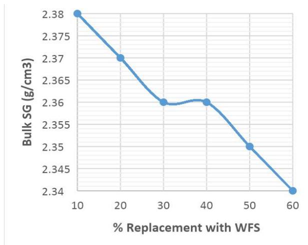
Figure 13: Bulk specific gravity (G) against different percentage replacement with WFS
