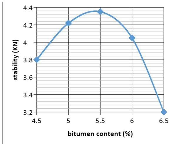
Figure 5: Stability against bitumen Content at 0% WFS
