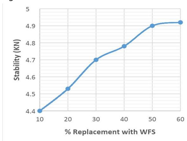
Figure 11: Stability against different percentage replacement of WFS
