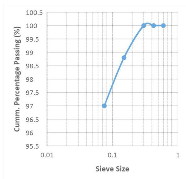
Figure 3: Sieve Analysis for Cement
