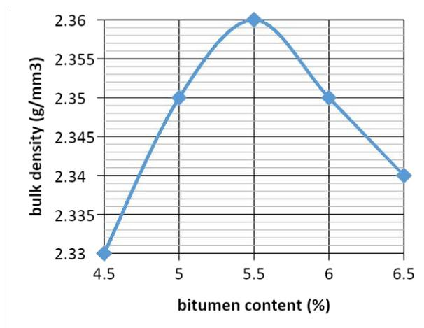
Figure 7: Bulk Density against Bitumen Content at 0% WFS
