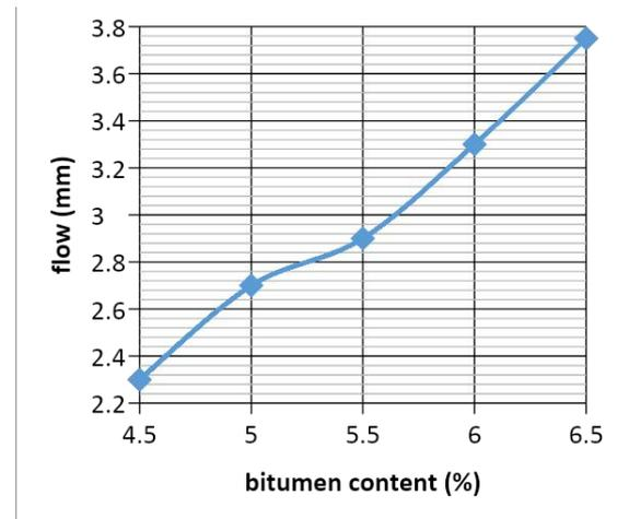
Figure 6: Flow against bitumen content at 0% WFS
