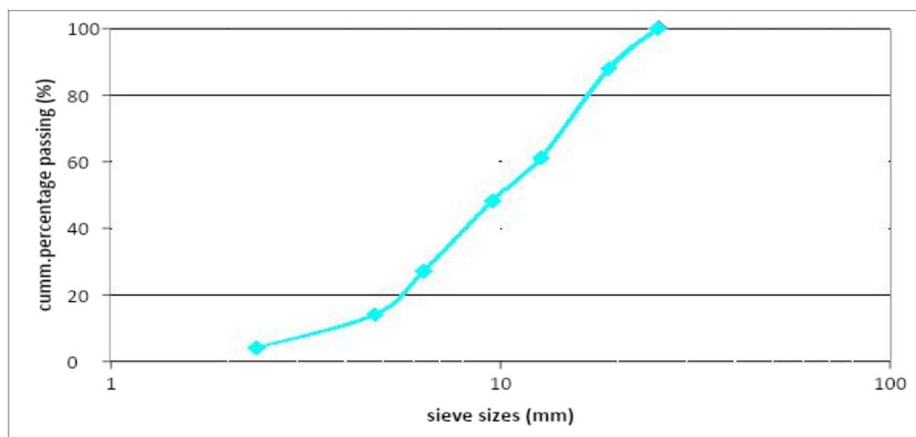
Figure 1: Sieve Analysis for Coarse Aggregate
