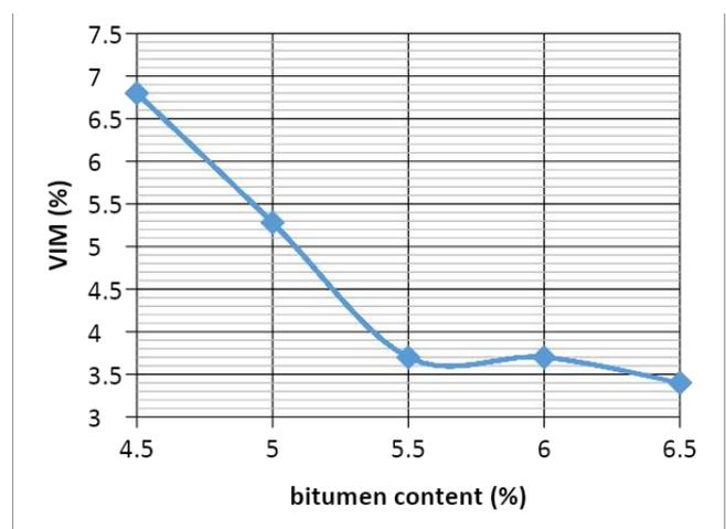
Figure 10: VIM against Bitumen Content at 0% WFS
