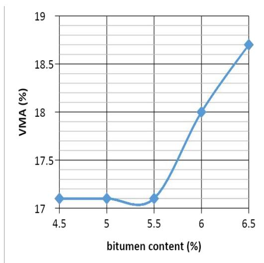
Figure 9: VMA against Bitumen Content at 0% WFS
