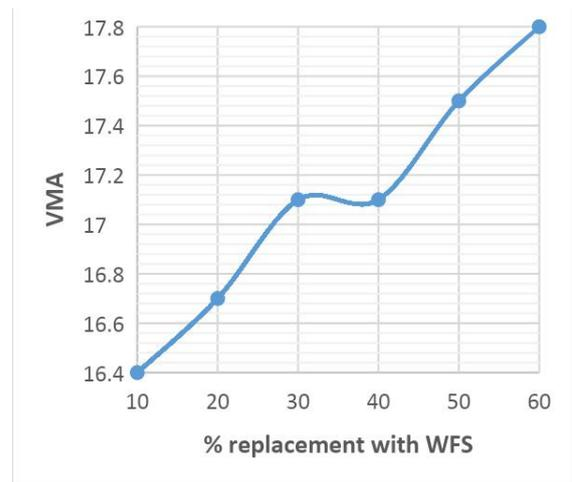
Figure 14: Void in mineral aggregates against different percentage replacement with WFS
