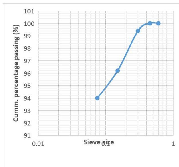
Figure 4: Sieve Analysis for Waste Foundry Sand
