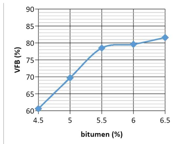
Figure 8: VFB against Bitumen Content at 0% WFS
