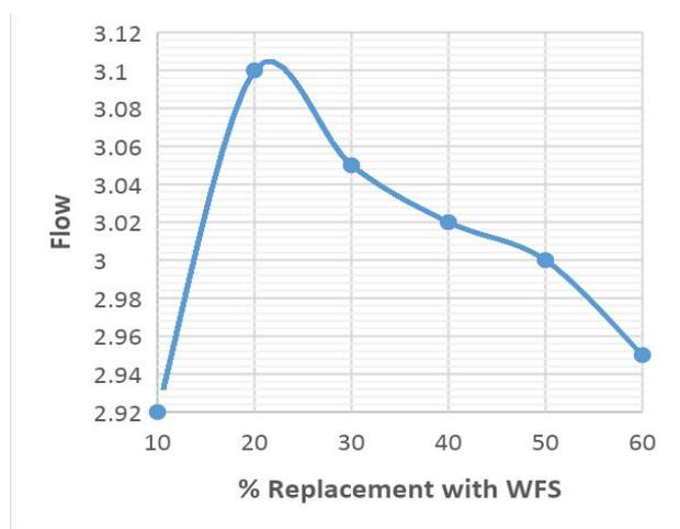
Figure 12: Flow against different percentage replacement of WFS
