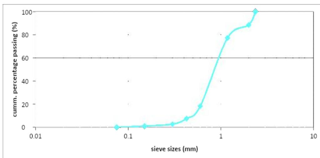
Figure 2: Sieve Analysis for Fine Aggregates
