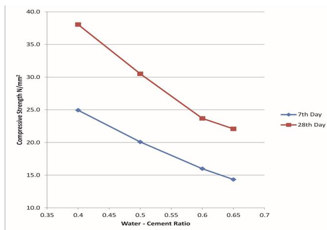
Figure 4: Compressive Strength at Various Water-Cement Ratio
