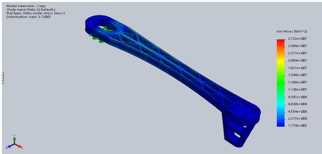
**Figure 2:** Maximum stress analysis of the arm.
