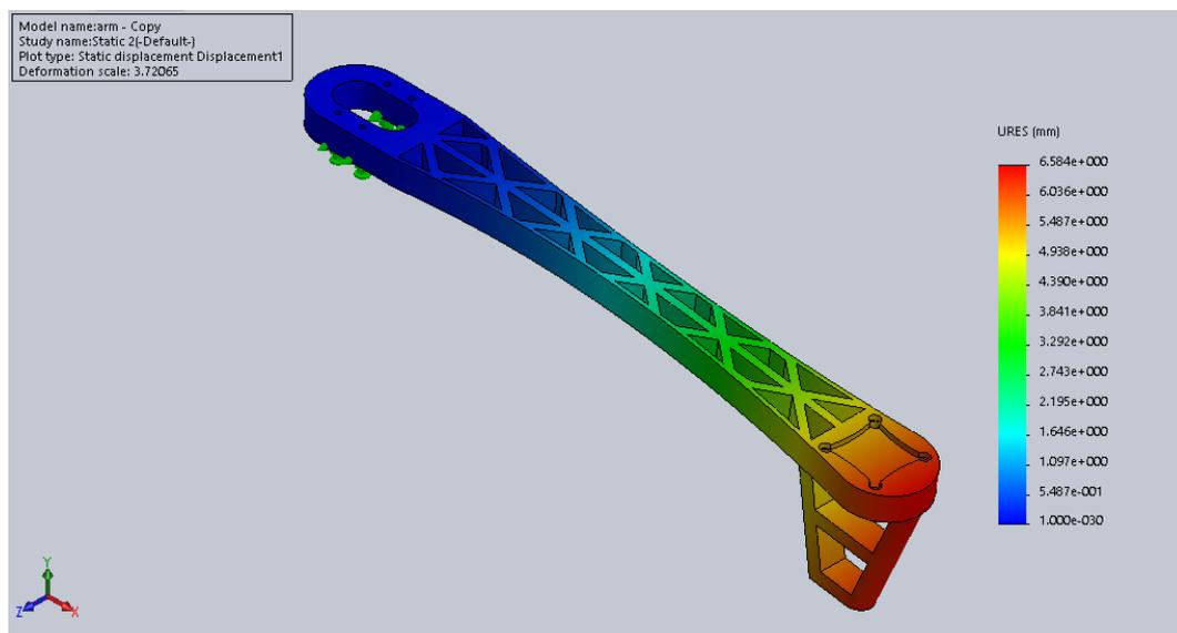
**Figure 3:** Maximum displacement of the quadcopter arm
