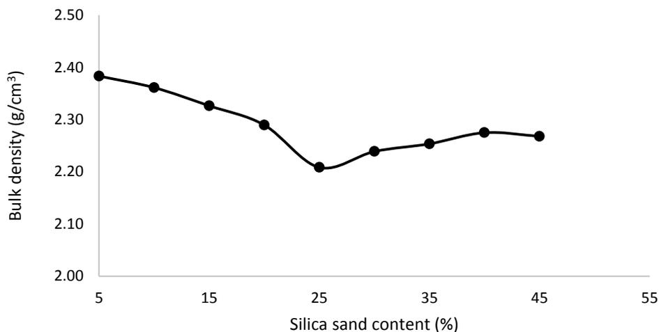
**Figure 6:** Variation of bulk density with silica sand content
