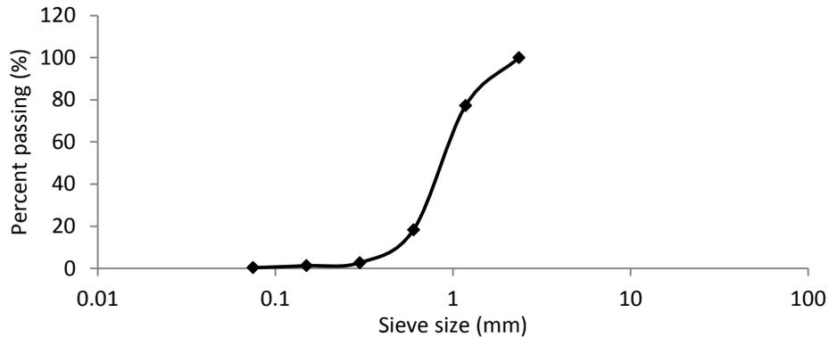
**Figure 2:** Particle size distribution curve for fine aggregate
