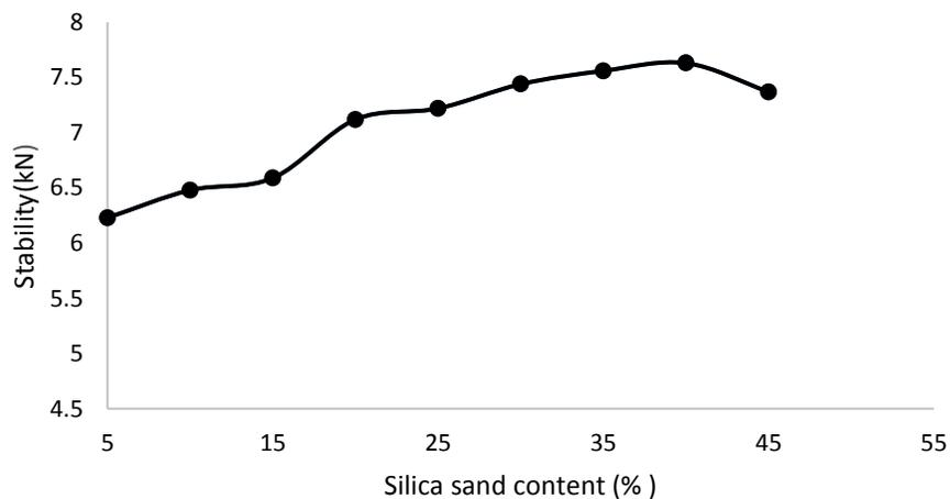
**Figure 3:** Variation of stability with silica sand content
