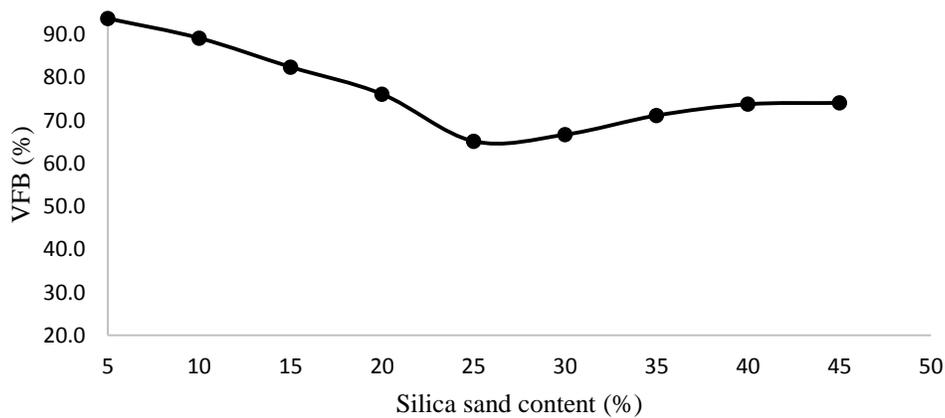
**Figure 7:** Variation of void filled with bitumen (VFB) with silica sand content
