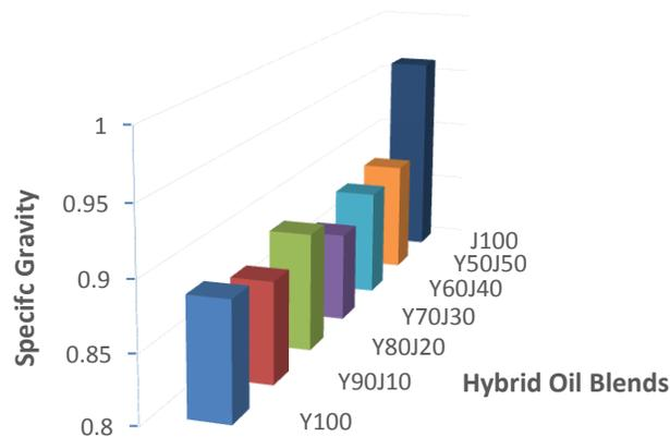
Figure 2: Influence of hybridization on specific gravity of hybrid methyl ester
