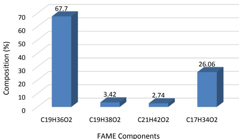
Figure 6: Chemical composition of Hybrid blend Y70J30 Biodiesel
