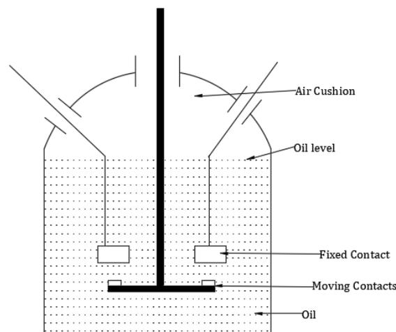
Figure 3: Oil circuit breaker (Bansal, 2019)
