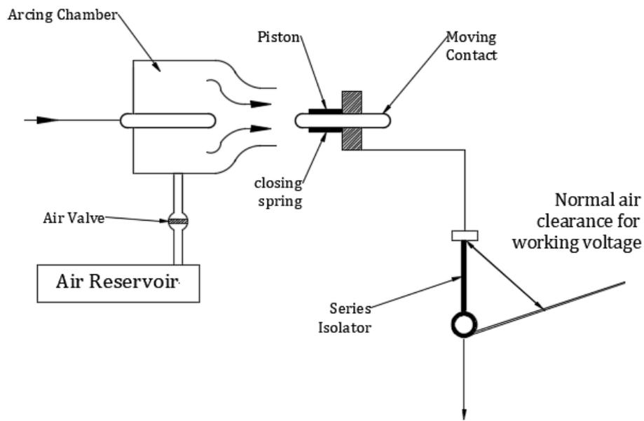
Figure 5: Air-blast circuit breaker (Goh et al., 2017)
