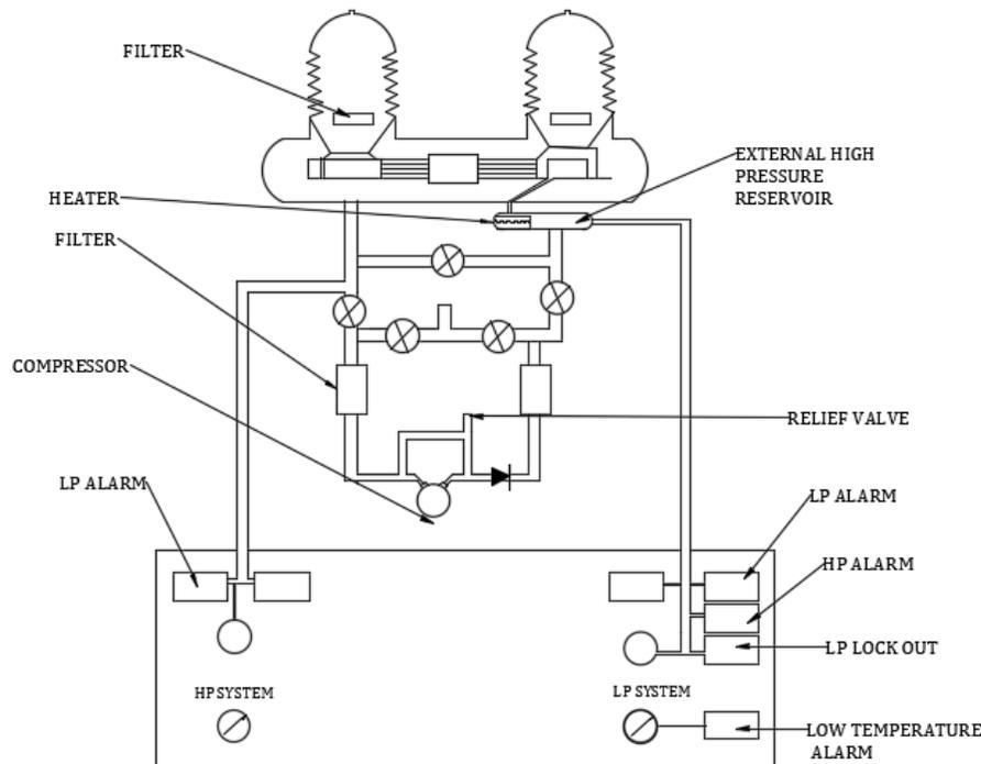
Figure 7: Sulphur hexafluoride circuit breaker (Wadhwa, 2012)
