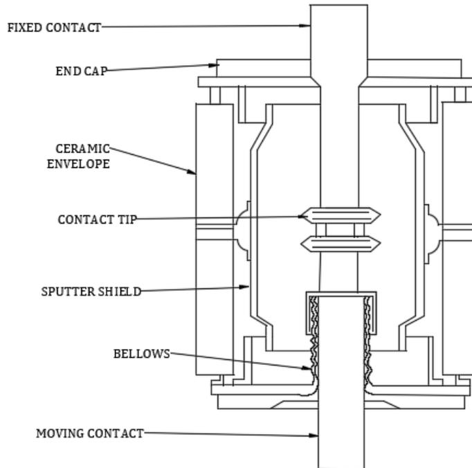
Figure 6: Vacuum circuit breaker (Gupta, 2015)
