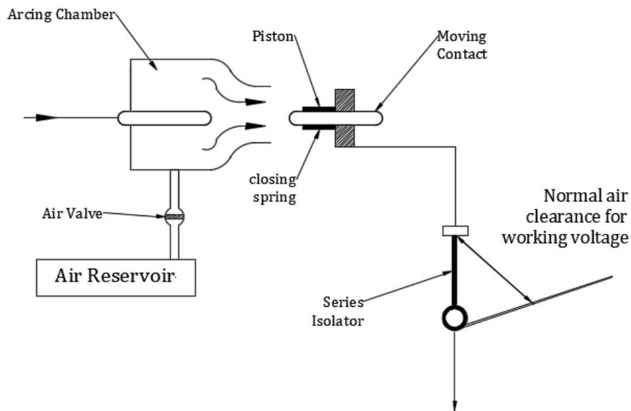
Figure 5: Air-blast circuit breaker (Goh et al., 2017)
