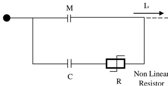
Figure 9: HVDC circuit breaker with non-linear resistance (Zheng *et al.*, 2019)
