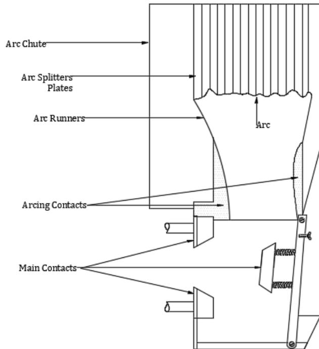
Figure 4: Air-break circuit breaker (Mehta and Mehta, 2008)
