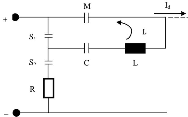
Figure 8: HVDC circuit breaker with series resonant L-C (Norum, 2016)
