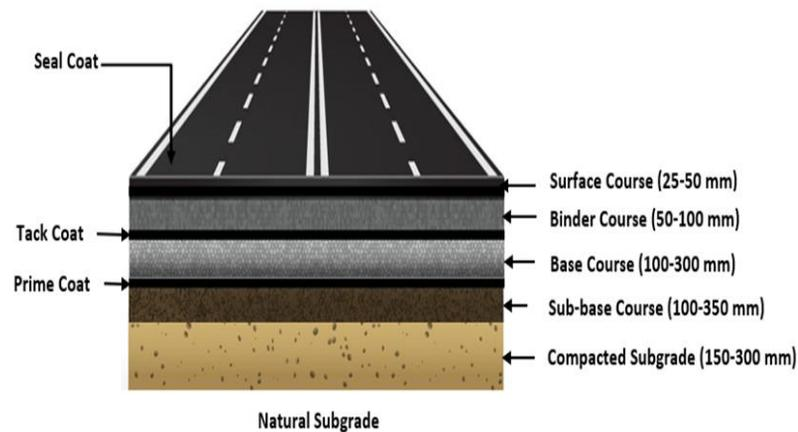
Figure 1: A Typical Flexible Pavement Structure (Note, 1993)
