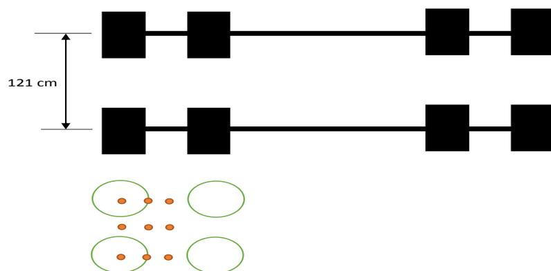
Figure 3: Standard Tandem Axle Load (Huang, 2004b)
