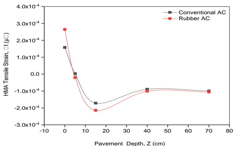
Figure 4: Computed Horizontal Tensile Strain
