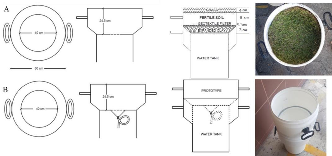
**Figure 2. A** Schematic drawing of the Prototype green roof and **B** the Pluviometer Prototype.
