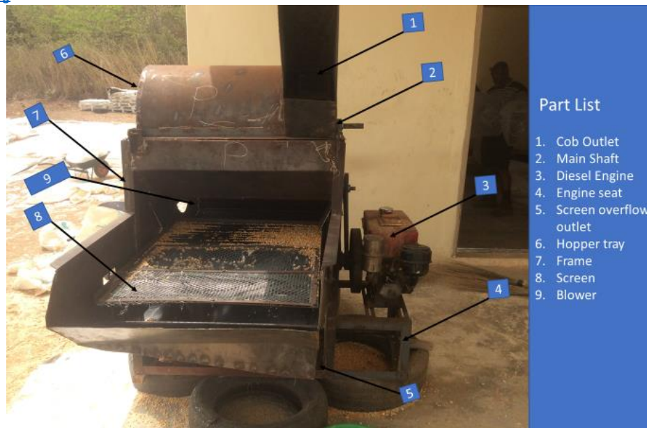
Figure 4. A multipurpose sheller
