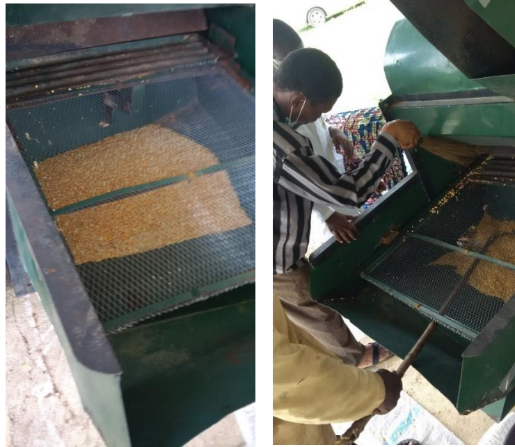
Figure 6: Heaping of grains at cleaning outlet
