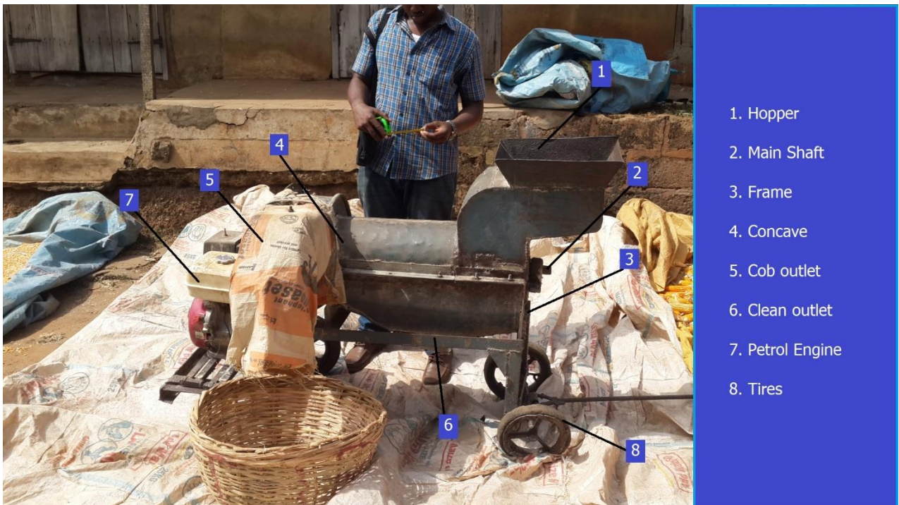
Figure 1. The basic maize sheller typically found in Nigerian markets
