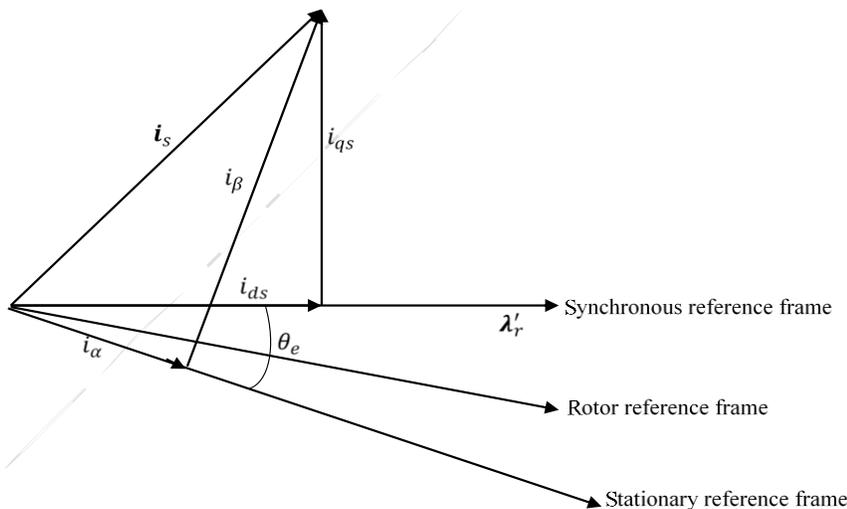
**Figure 2:** Rotor Flux Vector Alignment with the d-Axis
