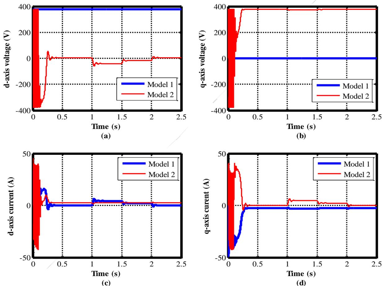
**Figure 7:** Simulation Results of d-q Axes Voltages and Currents
