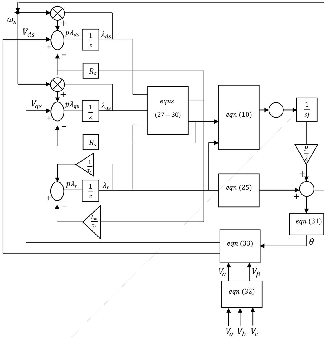
**Figure 5:** Block Diagram of the Solution to the Modified d-q Reference Frame Model (Model 2)
