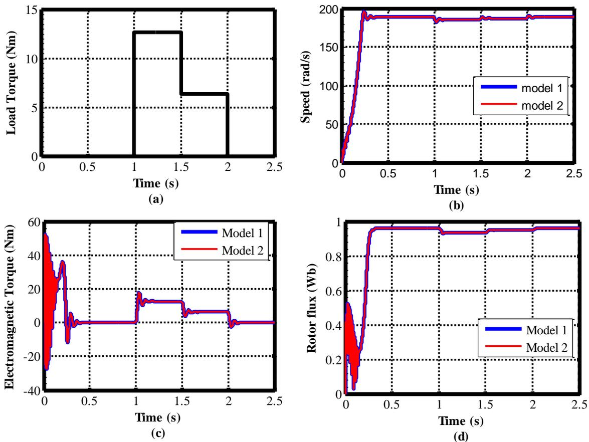
**Figure 6:** Simulation Results of Load Torque, Speed, Electromagnetic Torque and Rotor Flux
