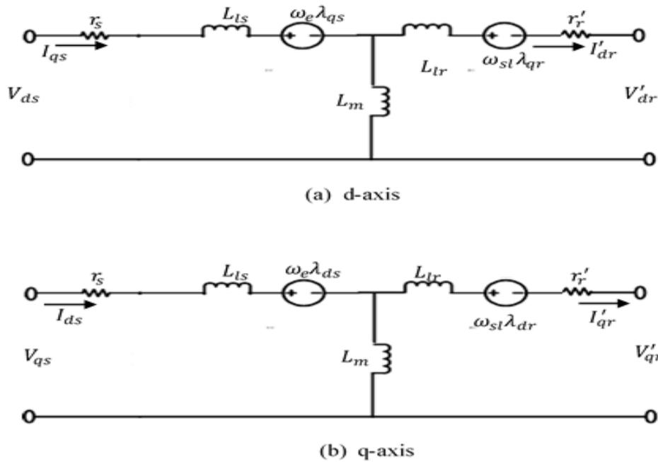
**Figure 1:** Equivalent circuit of the standard d-q reference frame model of the three phase Induction motor
