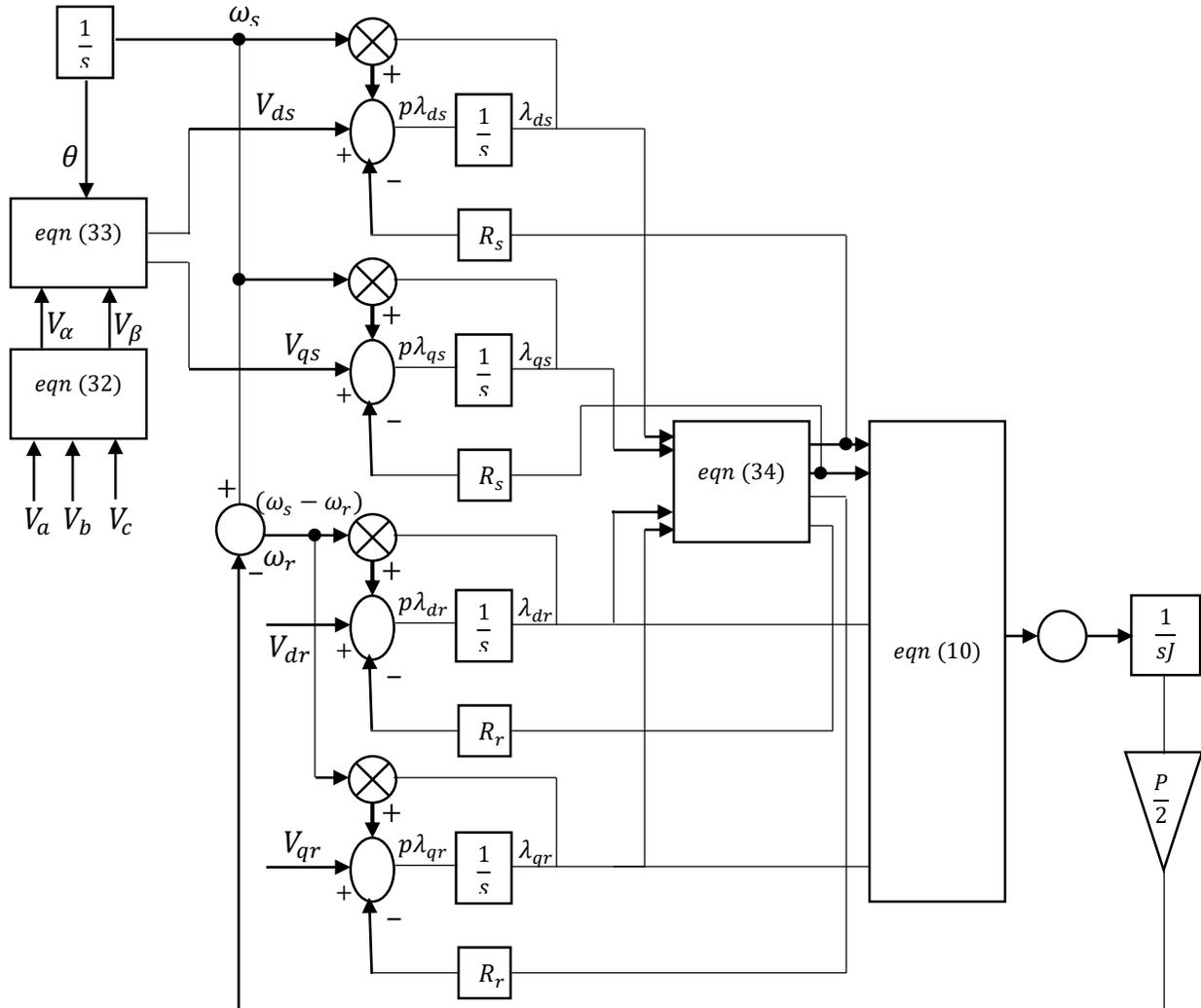
**Figure 4:** Block Diagram of the Solution to the Standard d-q Reference Frame Model (Model I)
