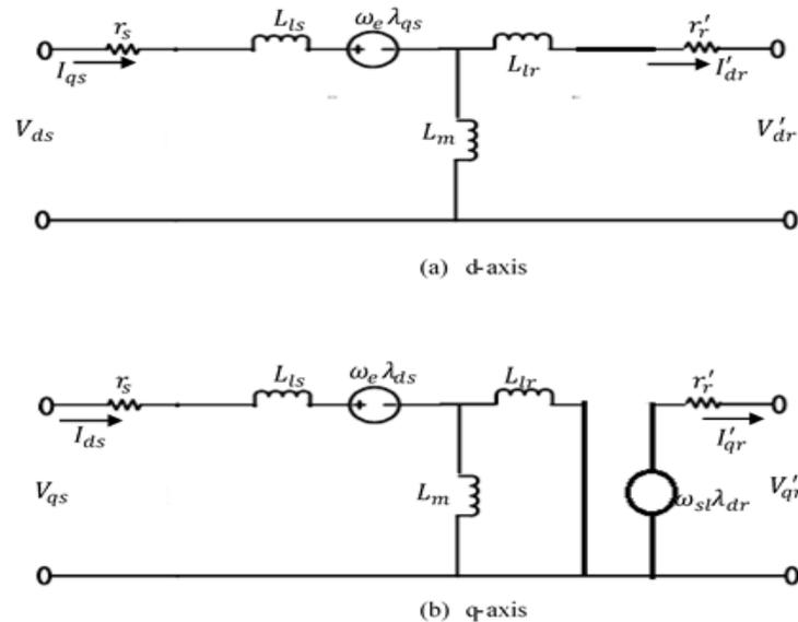
**Figure 3:** Equivalent circuit of the standard d-q reference frame model of the three phase Induction motor
