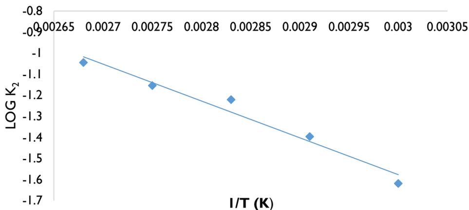
Figure 5 A plot of log of  $k_2$  against  $1/T(K)$  for bleaching process in the absence of Fe(III) ion
