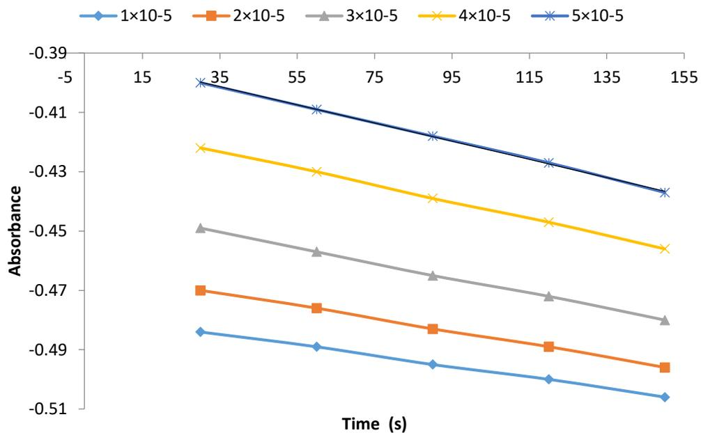
Figure 4 The Plot Log Abs against t for the effect of oxidant conc. on bleaching rate in the presence of Fe(III) ion
