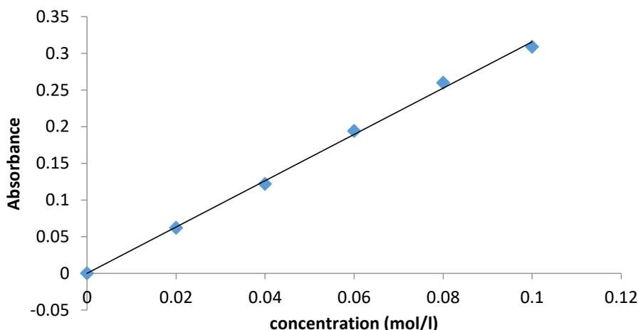
Figure 2: Plot of absorbance versus concentration for dye solution
