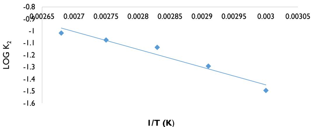
Fig. 6 A plot of  $k_2$  against  $1/T(K)$  for bleaching process in the presence of Fe(III) ion
