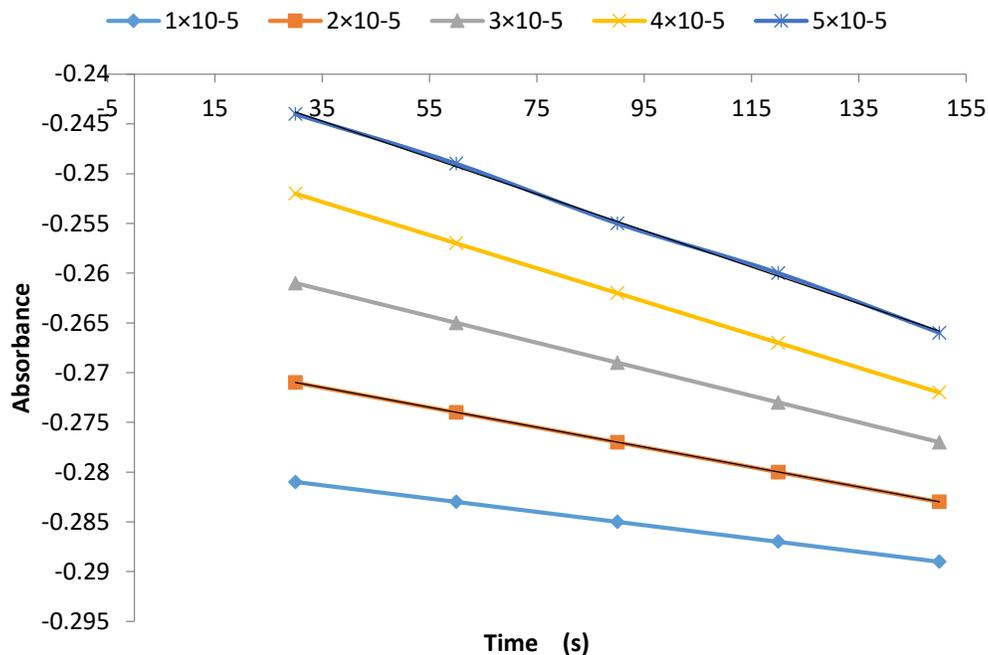
Figure 3 The Plot Log Abs vs t for the effect of oxidant conc. on bleaching rate in the absence of Fe(III) ion
