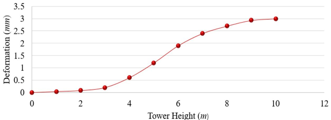
Figure 4. Deformation of the tower under the simultaneously predefined applied loads along its height.
