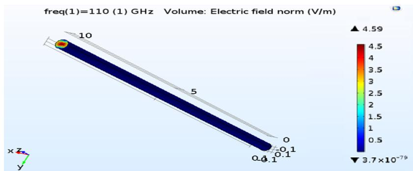
Figure 2. Frequency response of the transfer function in terms of electric field norm at 110 GHz excitation.
