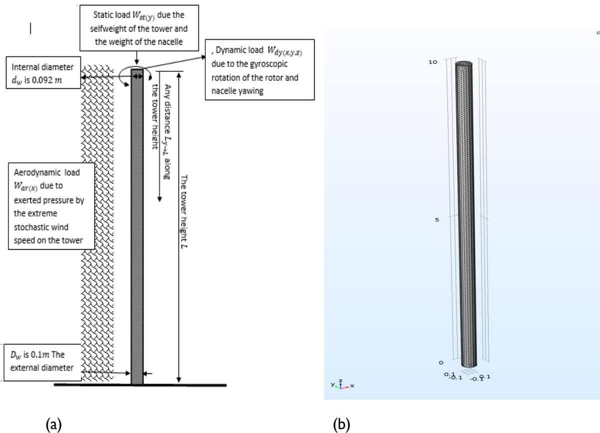
Figure 1: (a) Loads on the HAWT tower and (b) the generated grid.
