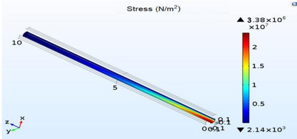
Figure 5. Stress distribution along the tower height due to simultaneously applied static, dynamic and aerodynamic loads.
