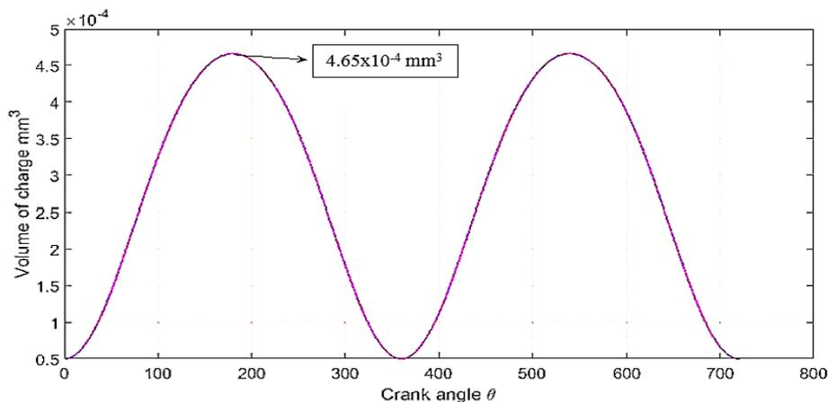
Figure 2: Plot of volume occupied by charge in cylinder against crank angle
