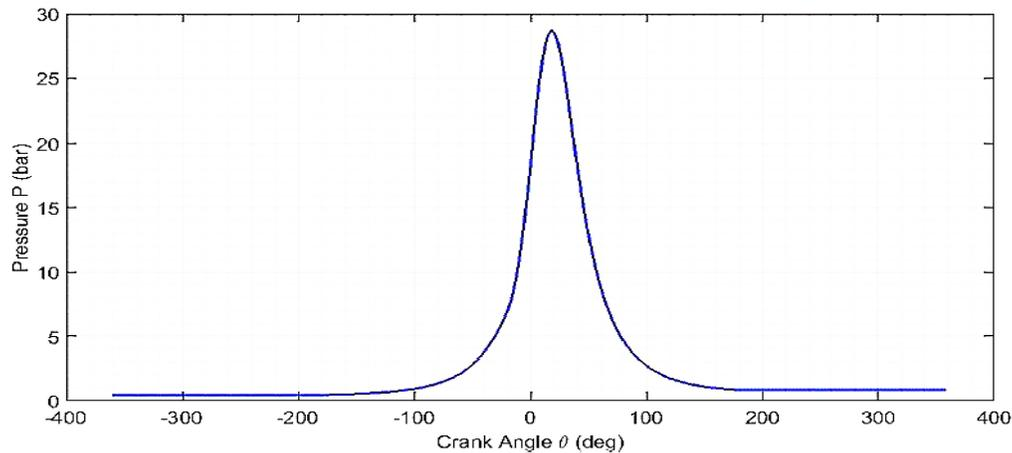
Figure 4: Plot of cylinder pressure against crank angle
