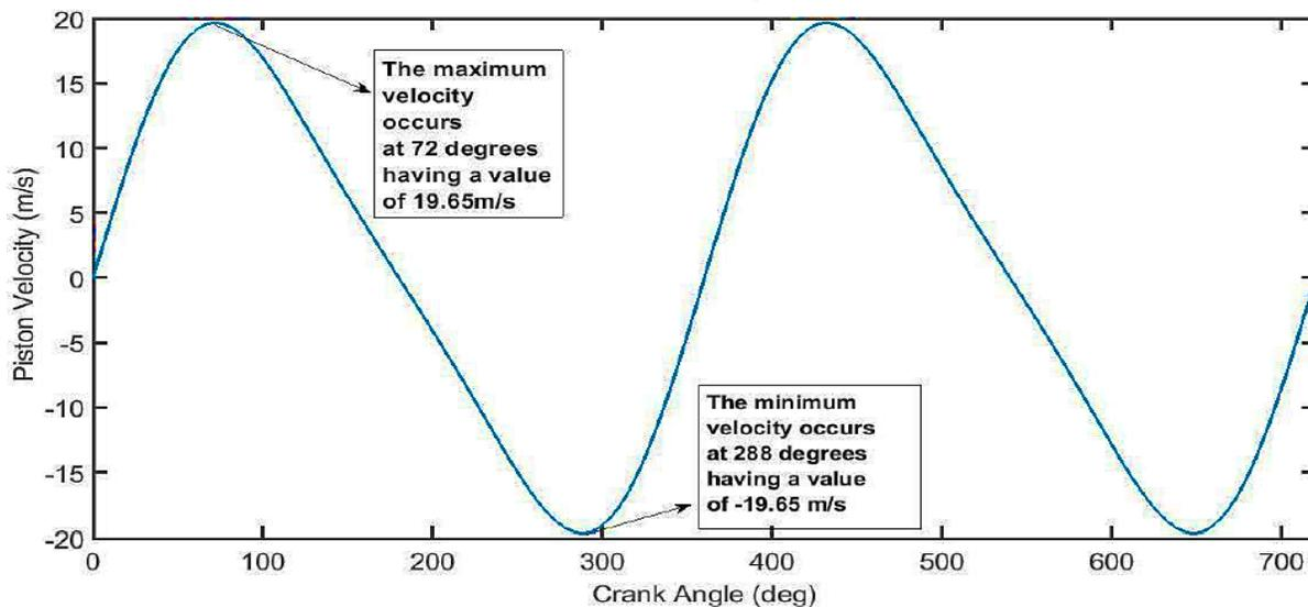
Figure 3: Plots of piston velocity against crank angle
