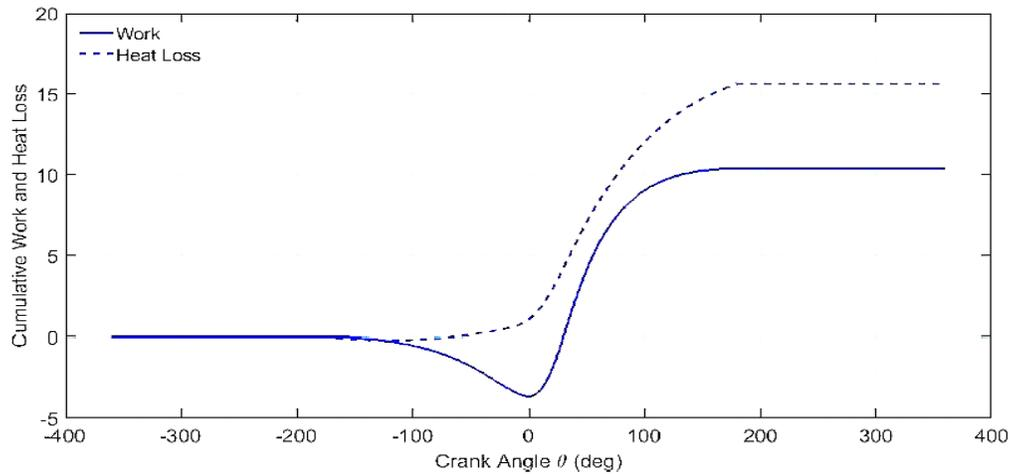
Figure 6: Plot of cumulative work and heat loss against crank angle
