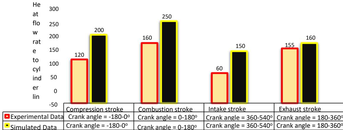
Figure 9: Heat flow rate to cylinder liner at different crank angles
