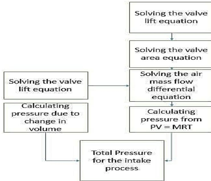
Figure 1: Flow chart for the intake process
