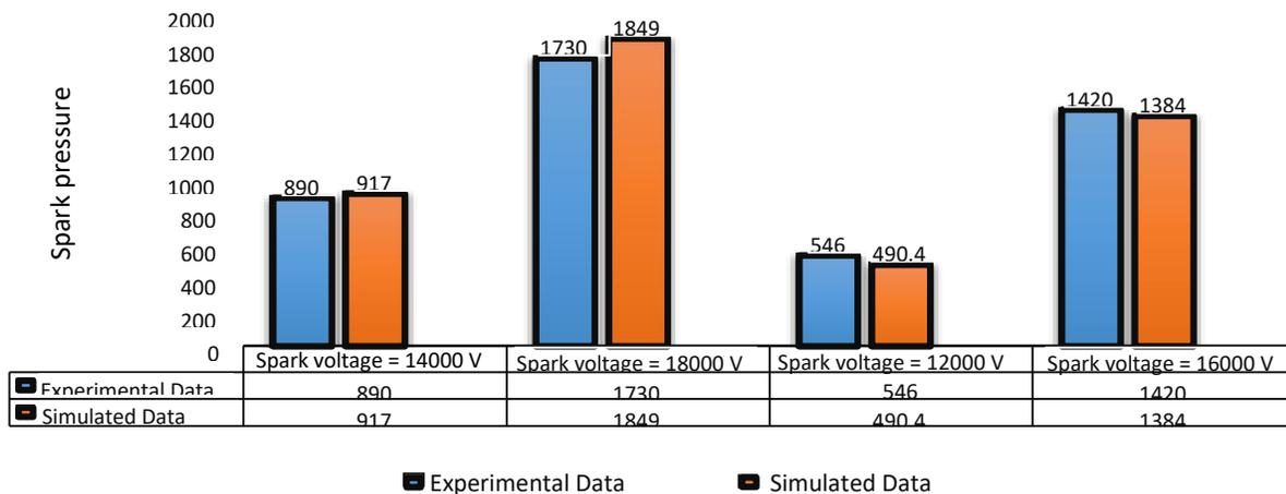
Figure 8: Spark pressure in cylinder before combustion for simulated and experimental data
