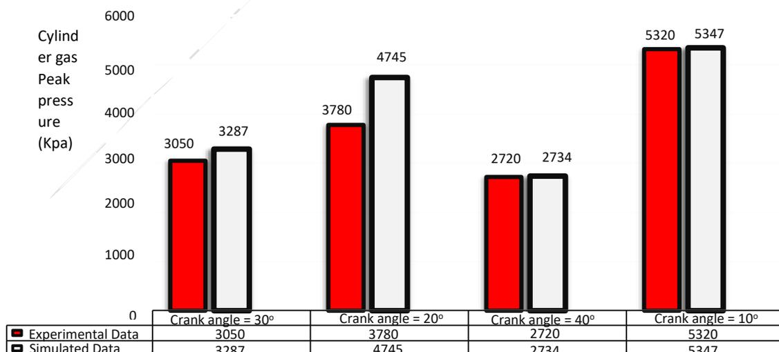
Figure 7: Peak pressure between simulated data and experimental data
