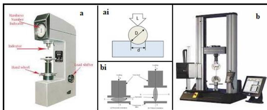
Figure 2. The Brinell Hardness Tester is shown in (a) and the test demonstration (ai). The Universal Testing Machine (b) demonstrating test of a specimen (bi)
