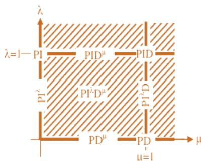
Figure. 1: FOPID Controllers Illustration
