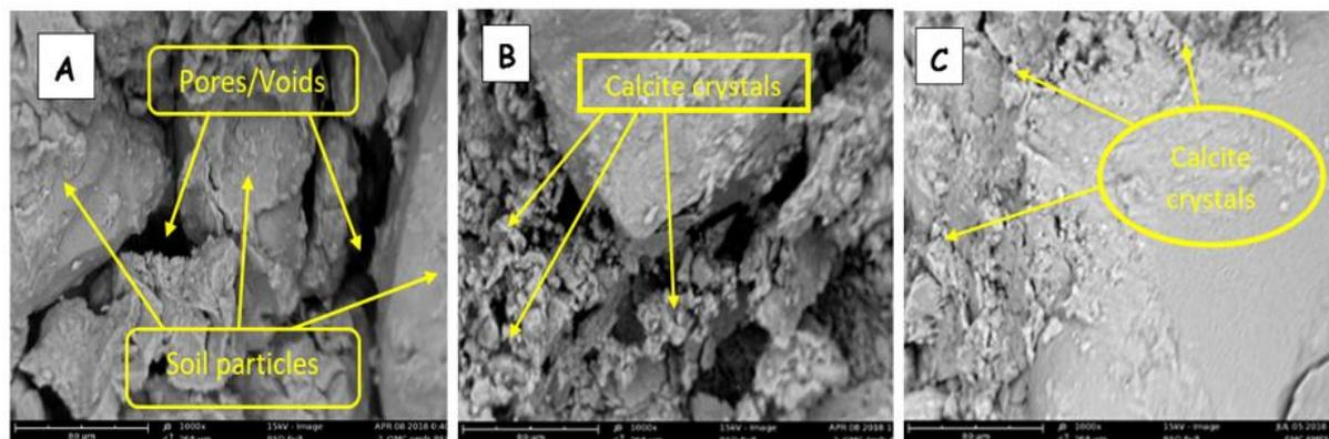
**Figure 7:** Micrograph at x1000 Magnification: (A) natural soil, (B) Unsterilized soil treated with  $1.20 \times 10^9$  cells/ml suspension density at -2% OMC, (C) Sterilized soil treated with  $1.80 \times 10^9$  cells/ml suspension density at OMC
