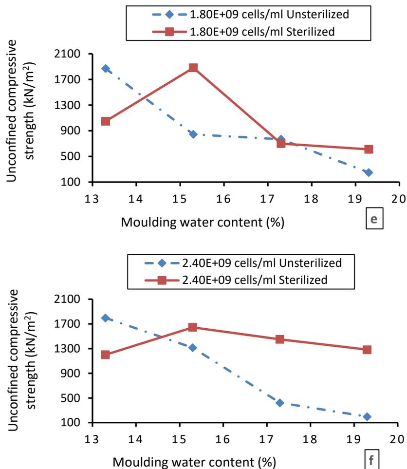
**Figure 6:** Variation of Unconfined compressive strength with moulding water content for Lateritic soil under sterilized and unsterilized condition, (a) natural soil, (b)  $1.50 \times 10^8$ , (c)  $6.0 \times 10^8$ , (d)  $1.20 \times 10^9$ , (e)  $1.80 \times 10^9$  and (f)  $2.40 \times 10^9$ /ml *S. pasteurii* suspension densities
