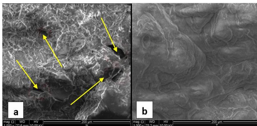
**Figure 8:** Micrograph at x1000 Magnification of samples for Atterberg limits: (a) natural soil, (b) Unsterilized soil treated with  $1.20 \times 10^9$  cells/ml suspension density at -2% OMC
