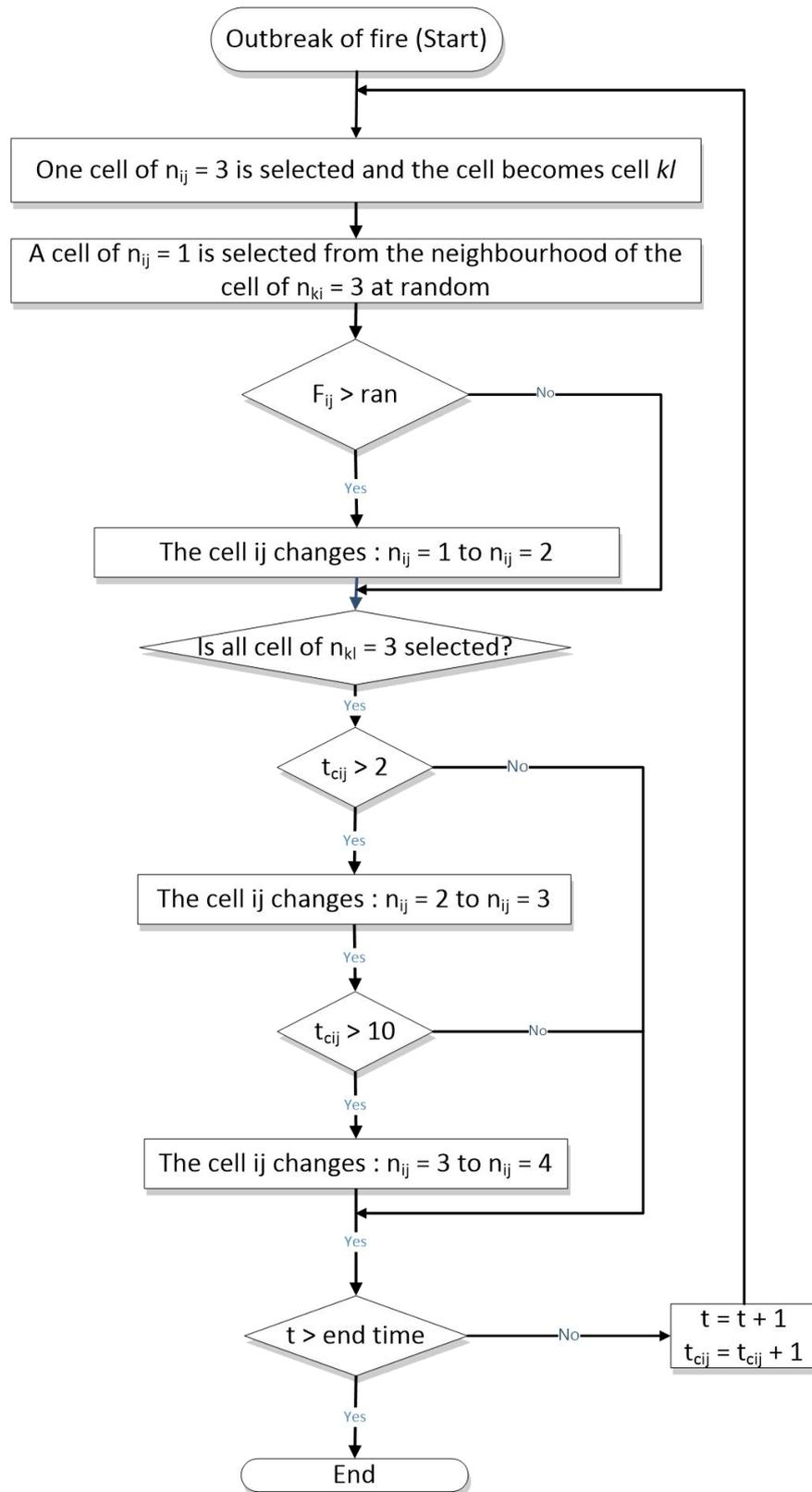
Figure 3: Flow chart of the fire spread model
