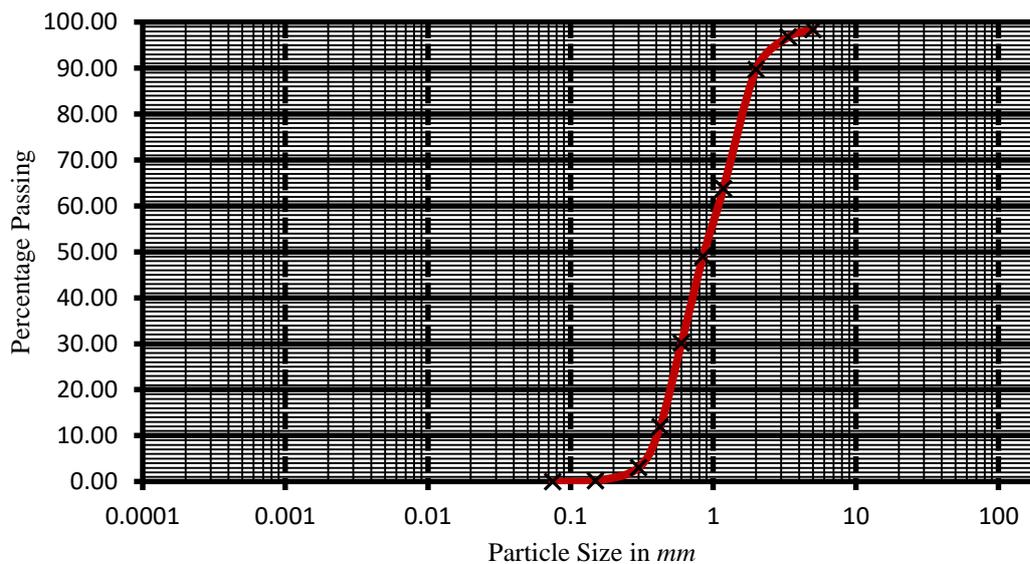
**Figure 1:** Particle- Size Distribution Curve for the Sand
