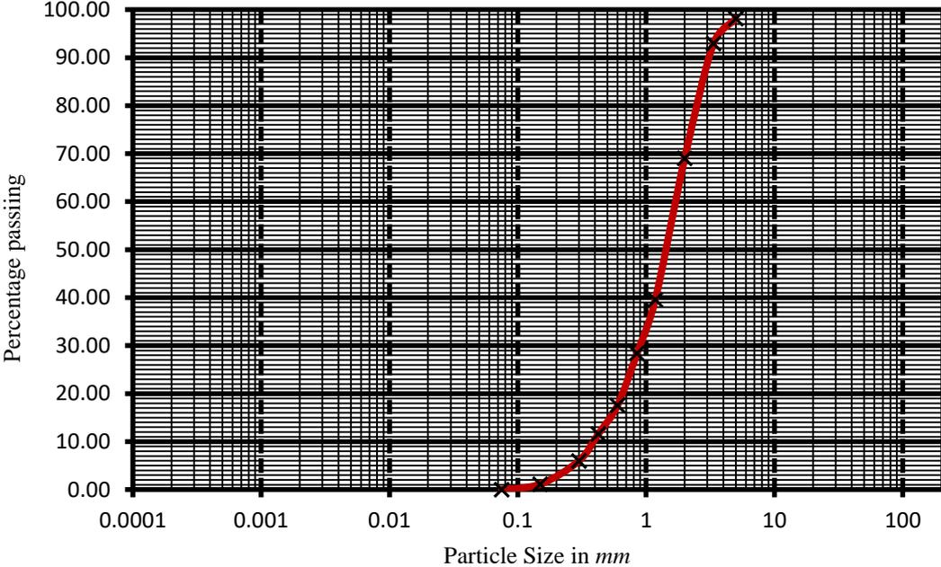
**Figure 2:** Particle-Size Distribution Curve of the SRMW
