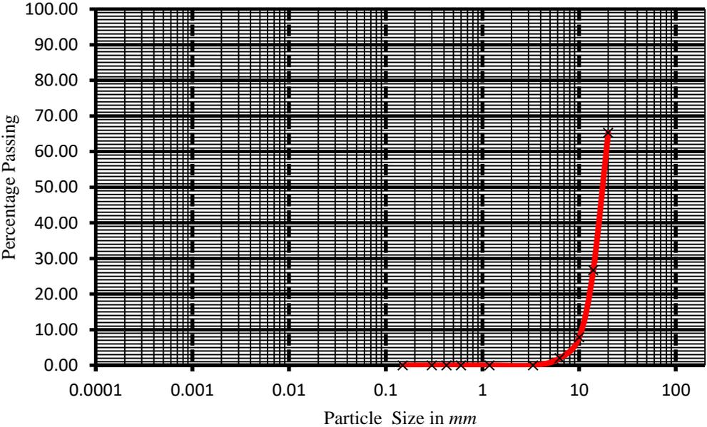
**Figure 3:** Particle-Size Distribution Curve of the Coarse Aggregate
