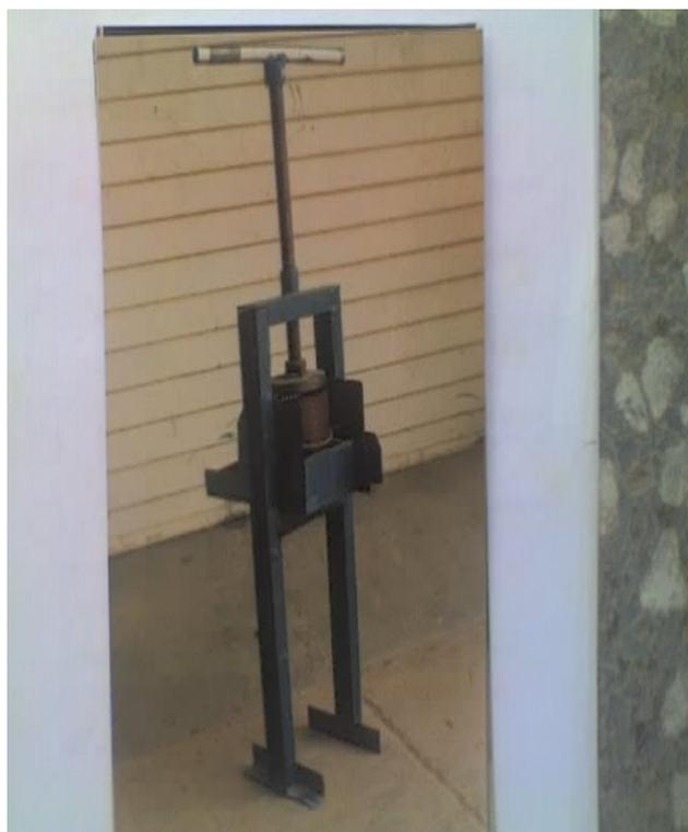
**Figure 1: Photograph of the spindle oil press**
