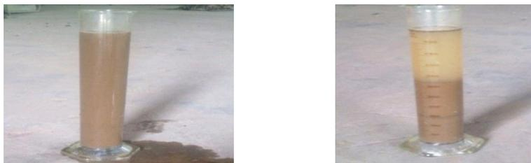
Figure 1: Measuring of Clay Content
