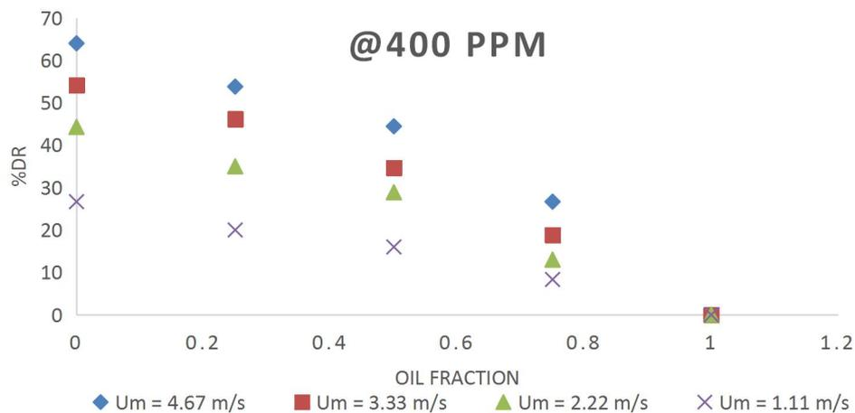
Figure 3: Effect of oil fractions on drag reduction at various mixture velocities (horizontal flow)
