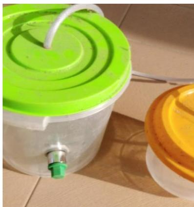
Figure 3: The Digester showing the male female socket
