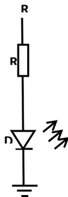
Figure 5: The Series connection between The Miniature Indicator Light Emitting Resistor and a Ballast Resistor.
