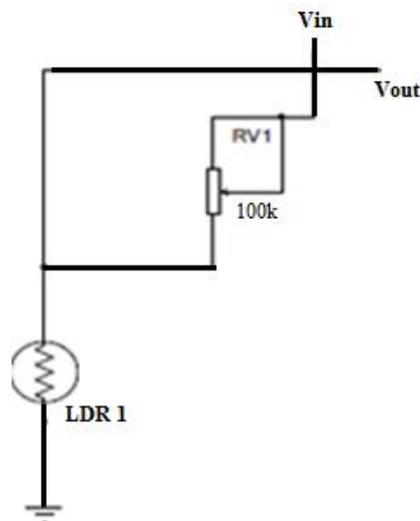
Figure 4: Voltage Divider between LDR and Potentiometer.
