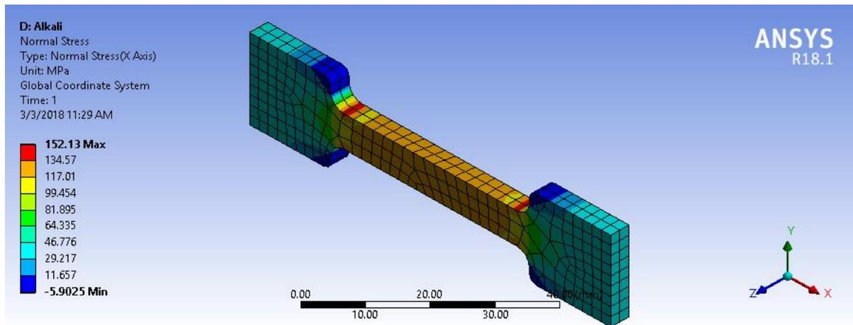
**Figure.7:** Contour Plots Showing Regions of Stress Concentration for Alkali Treated Fibres
