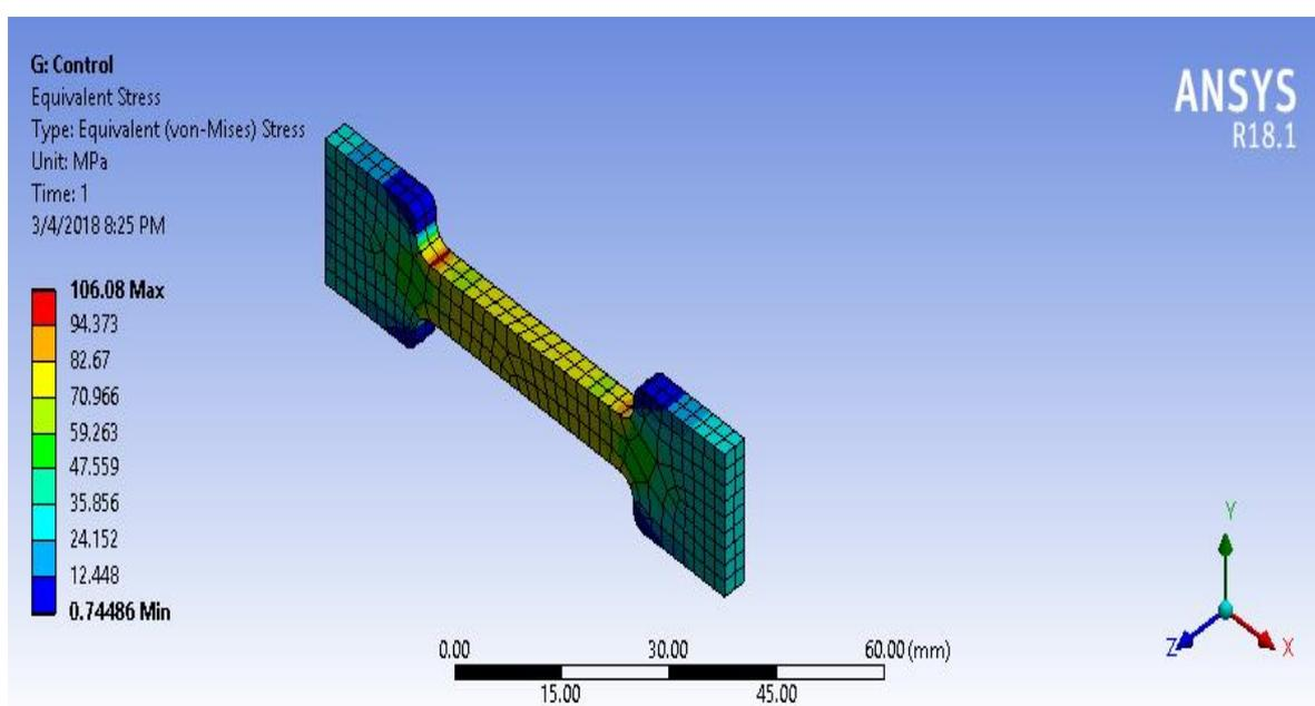
**Figure. 5:** Contour Plots Showing Regions of Stress Concentration for Untreated Fibres
