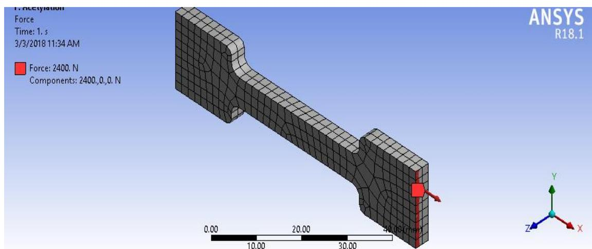
**Figure 3:** Boundary condition and load applied for ANSYS work bench model
