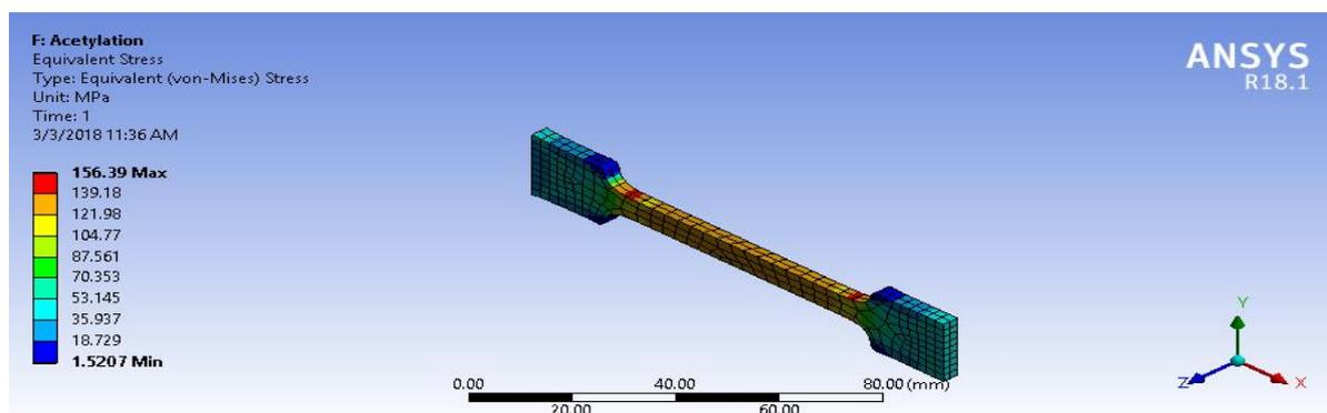
**Figure. 6:** Contour Plots Showing Regions of Stress Concentration for Acetylation Treated Fibres
