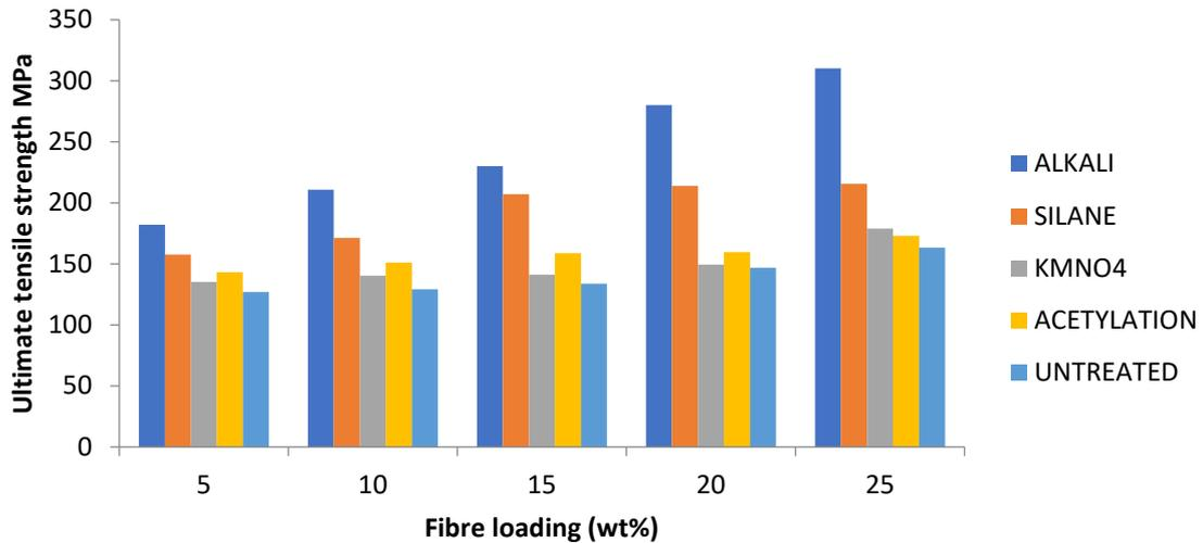
**Figure 4:** Influence of Surface Treatment and Fibre Composition on Tensile Strength of Composites
