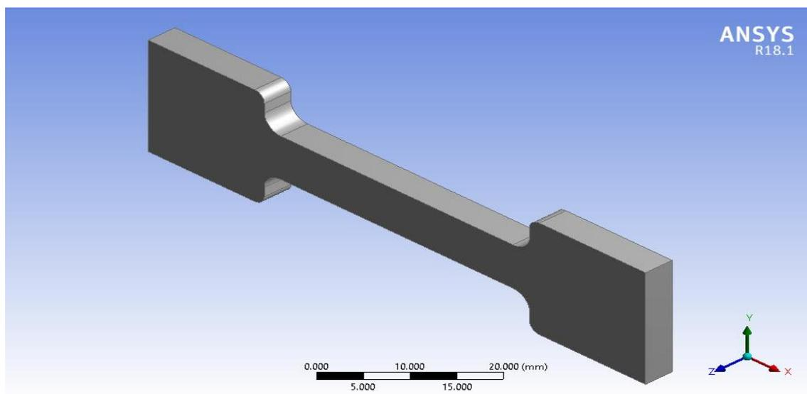
**Figure 2:** Geometry of tensile simulation specimen on ANSYS workbench
