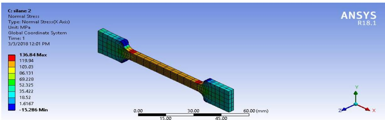
**Figure. 9:** Contour Plots Showing Regions of Stress Concentration for Silane Treated Fibres
