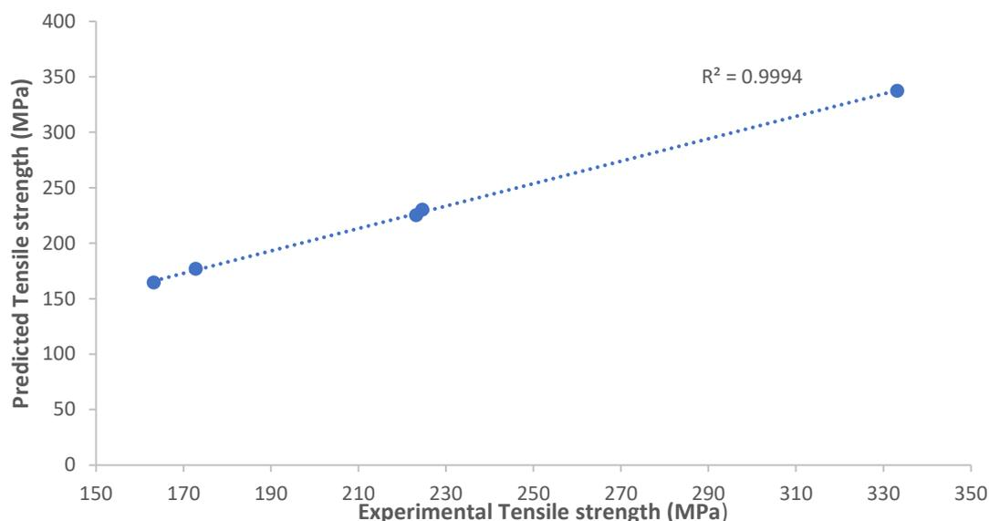
**Figure. 10:** Correlation of Predicted with Experimental Tensile Strength using Finite Element Modelling
