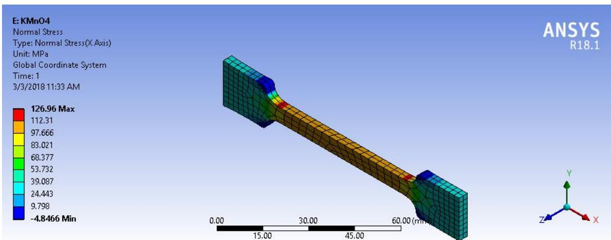
**Figure. 8:** Contour Plots Showing Regions of Stress Concentration for  $\text{KMnO}_4$  Treated Fibres
