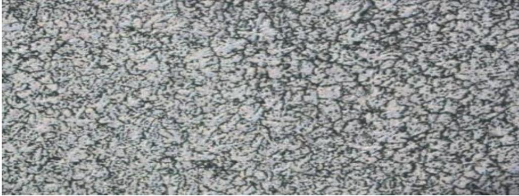
**Figure 7:** Microstructure of weld metal (x100)
