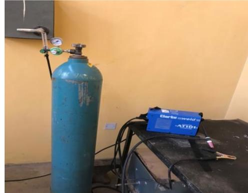
**Figure 3:** Tungsten inert gas welding setup
