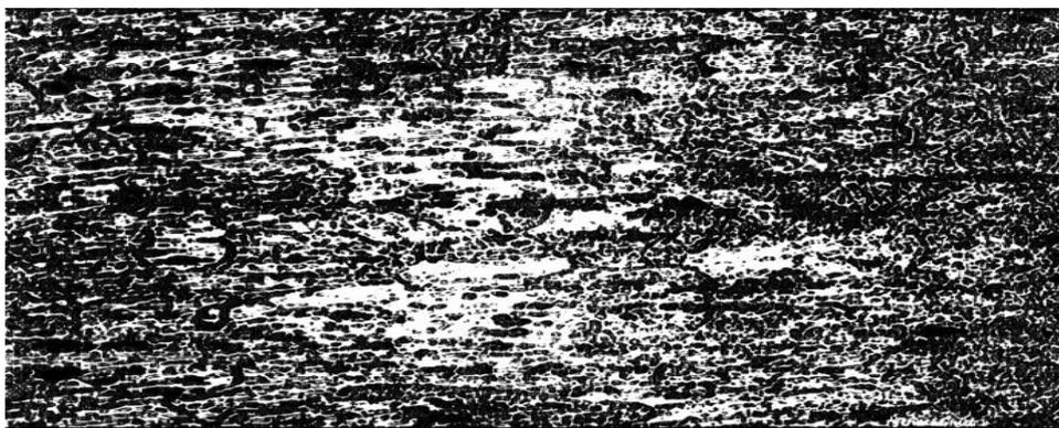
**Figure 6:** Microstructure of unwelded Aluminium 6061 (parent metal) (x100)
