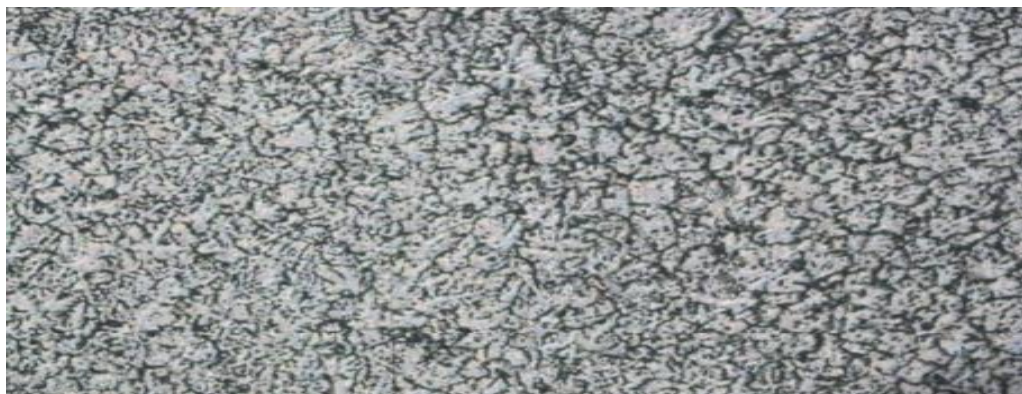
Figure 7: Microstructure of weld metal (x100)
