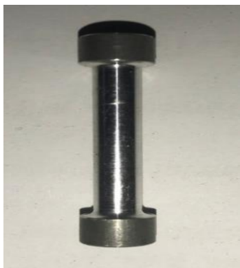
Figure 2: Aluminium 6061 tensile test specimen as per ASTM standard
