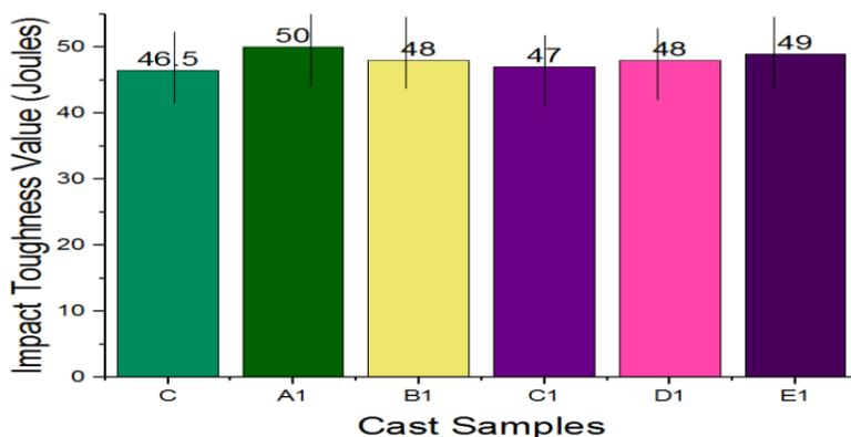
Figure 15: Variation of the Impact Toughness Values of the cast samples with wt%Sb for 1 hour austempering time for an Austempering Temperature of 300°C
