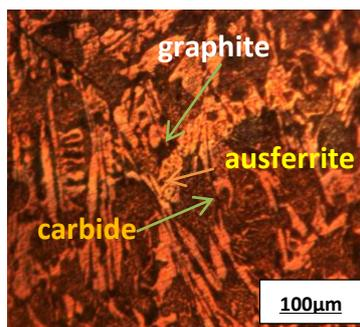
Figure 2: 0.12 %wt. Sb at 300 °C
