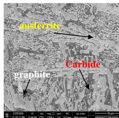
Figure 9: 0.24 % wt. Sb at 300 °C
