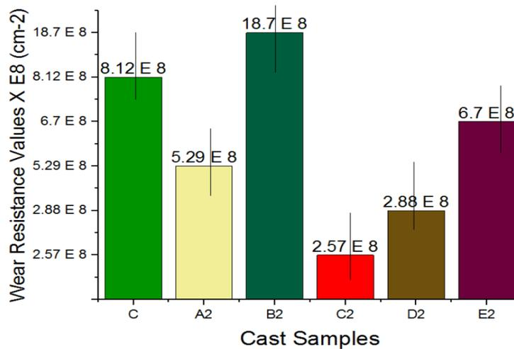
Figure 14b: Variation of the Wear Resistance Values of the cast samples with wt%Sb for 2 hours austempering time for an Austempering Temperature of 300°C
