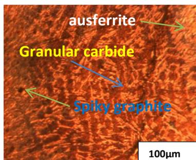
Figure 5: 0.41 % wt. Sb at 300 °C
