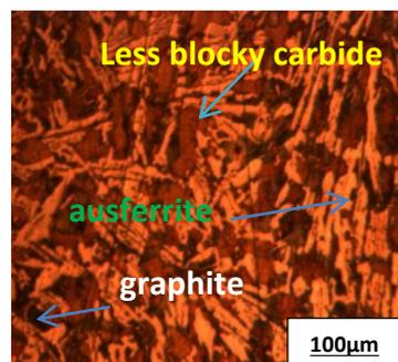
Figure 3: 0.24 % wt. Sb at 300 °C
