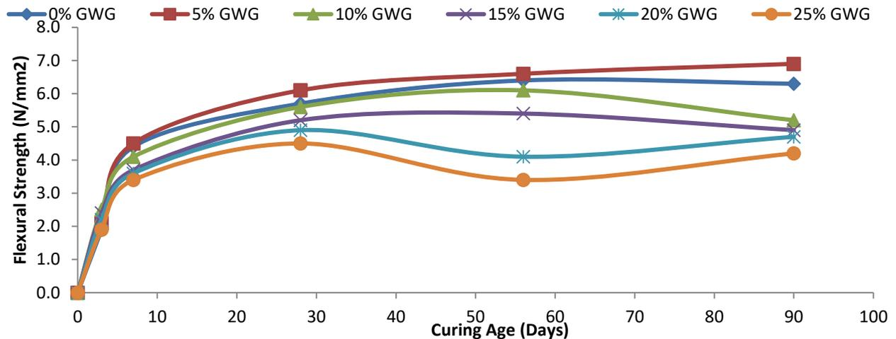
**Figure 5.** Flexural Strength of GWG-HPC
