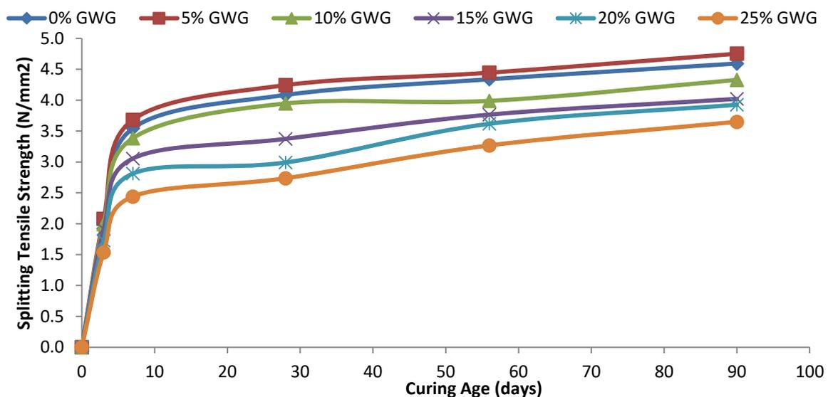
**Figure 4.** Splitting Tensile Strength Development of GWG-HPC
