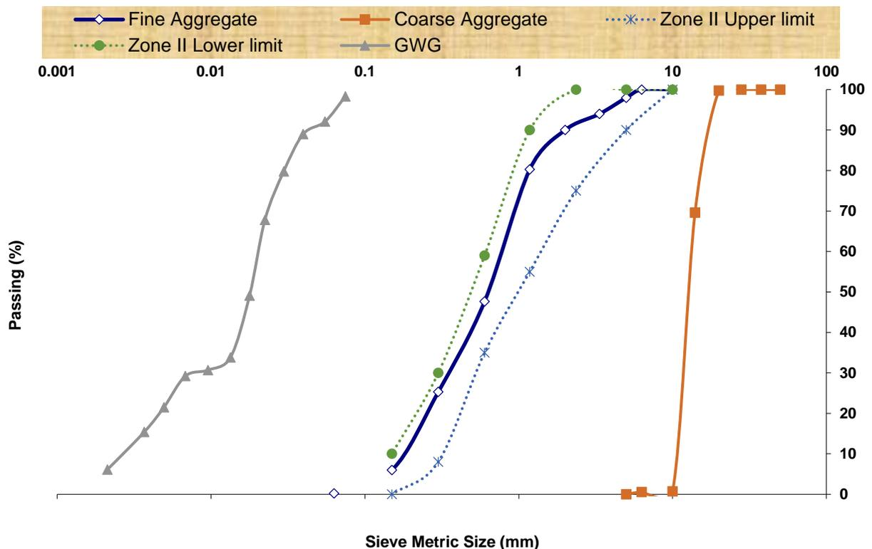
**Figure 1.** Particle size distribution chart of GWG, fine and coarse aggregates
