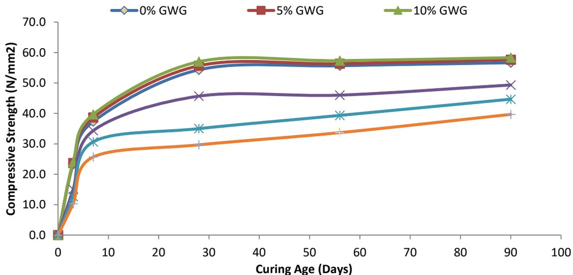
**Figure 3.** Compressive Strength of GWG-HPC.
