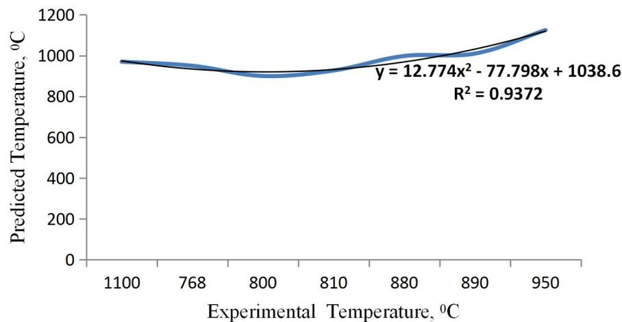
Figure 4: Experimental and CFD Predicted results validation
