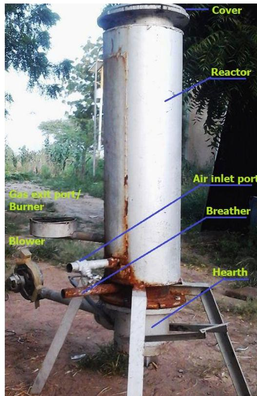
Figure 1: Downdraft Gasifier facility developed by Abubakar (2013)
