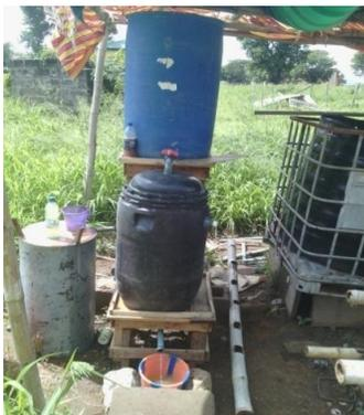
**Figure 1:** Sand filter treatment for poultry waste
