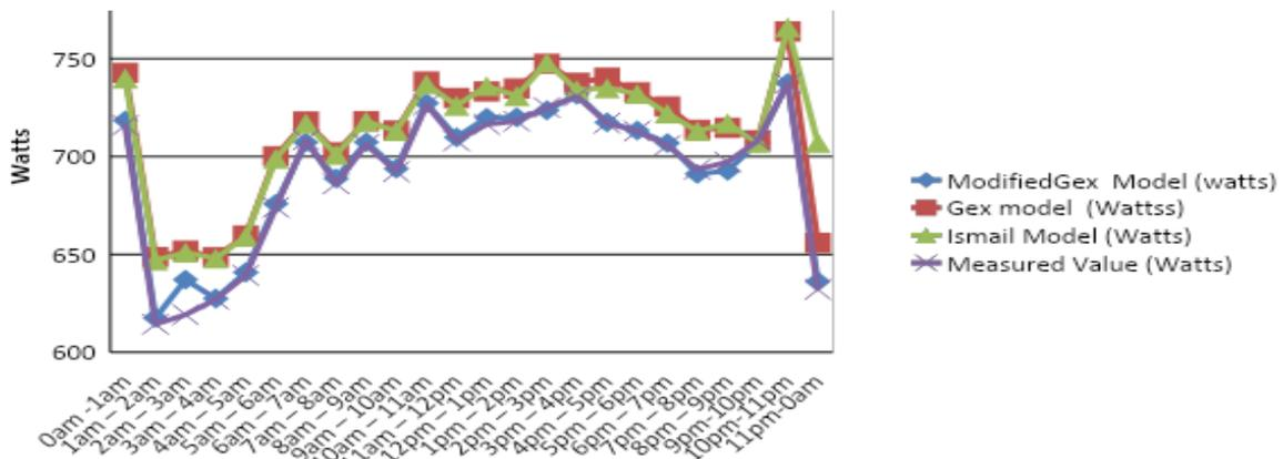
**Figure 2:** Comparison of the measured values with Gex model modified Gex model and Ismail model for micro cell base station
