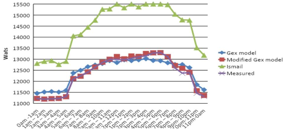
**Figure 1:** Comparison of the measured values with Gex model, modified Gex model and Ismail model for macro cell base station
