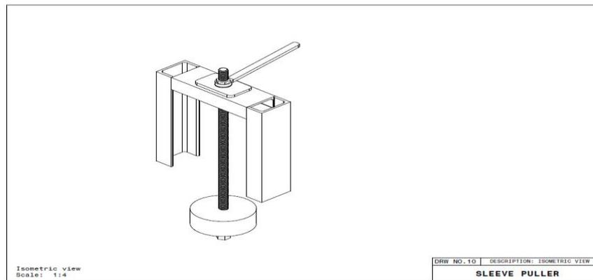
**Figure 3** Assembled sleeve puller (Isometric view)
