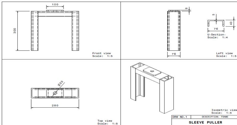
**Figure 1:** Sleeve puller frame
