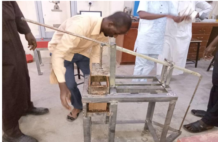
Figure 8: Demoulding lateritic earth block using the demoulder designed and fabricated by the author
