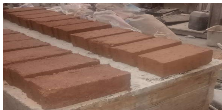
Figure 9: Lateritic earth blocks in an open-air for drying
