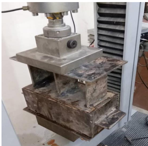
Figure 6: Compressing CLEB using UTM Figure 7: Isometric drawing of UTM Machine
