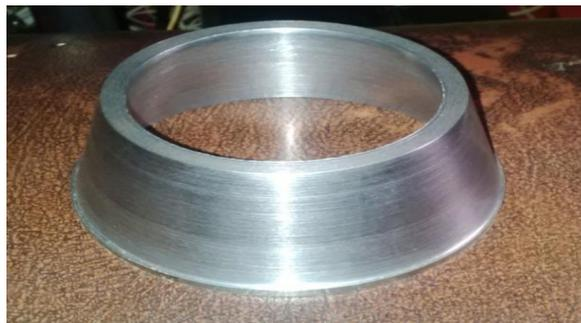
Figure 2.3: Mortar Flow Mould
