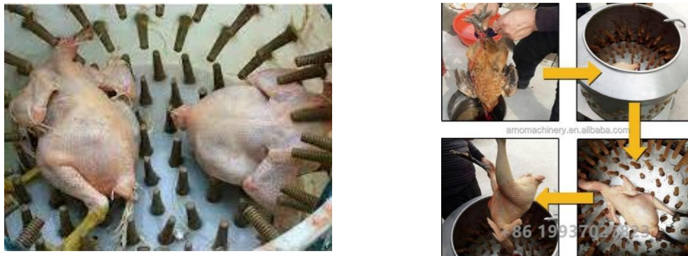
Figure 3: Mechanical Chicken Feather Plucking Machine (farmsquare, 2021)
