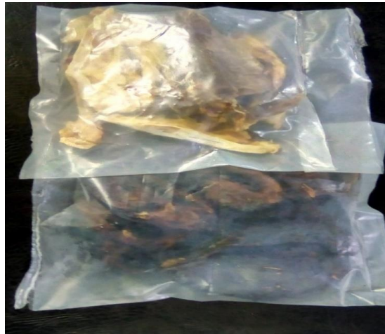
Figure 4: Vacuum Packaged Cat Fish and Cod Fish (Stock Fish) in Produced Polypropylene Packaging Films
