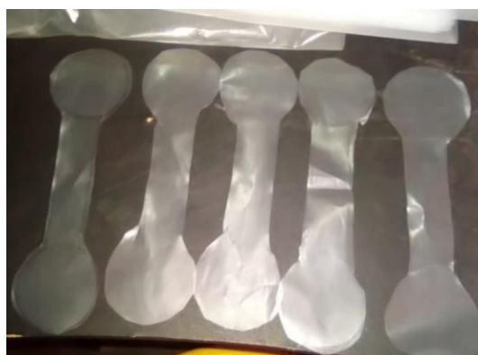
Figure 3: Dumb bell-shaped specimen from a set of samples of Produced polypropylene film ready for testing
