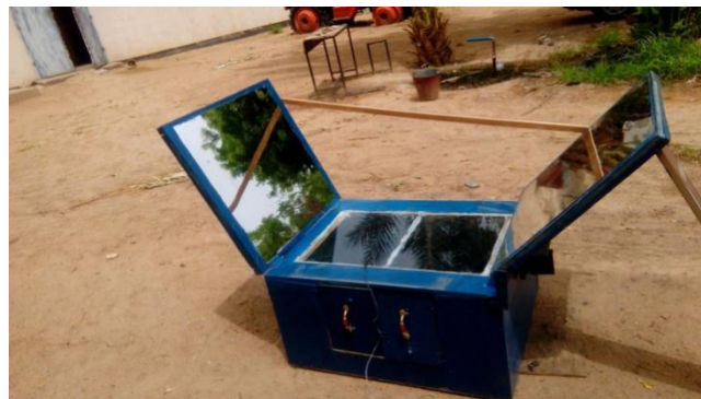
Figure 1: Double Compartment Solar Box Cooker (DCSBC)
