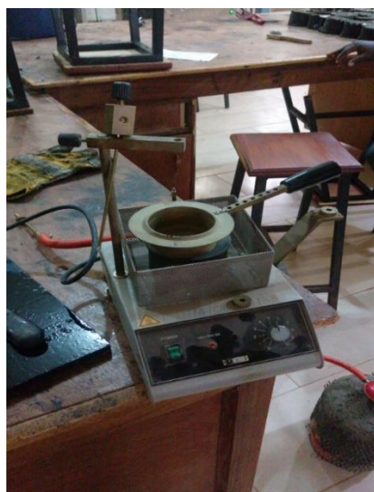
Figure 5: Flash and Fire Point Test Apparatus
