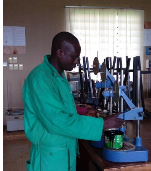
Figure 2: Penetration test Set-up
