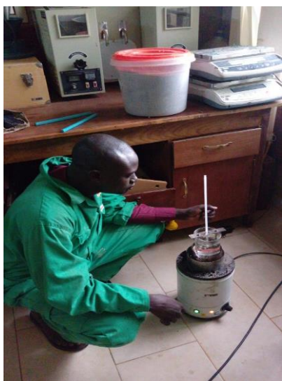
Figure 4: Ring and Ball Softening Point Apparatus
