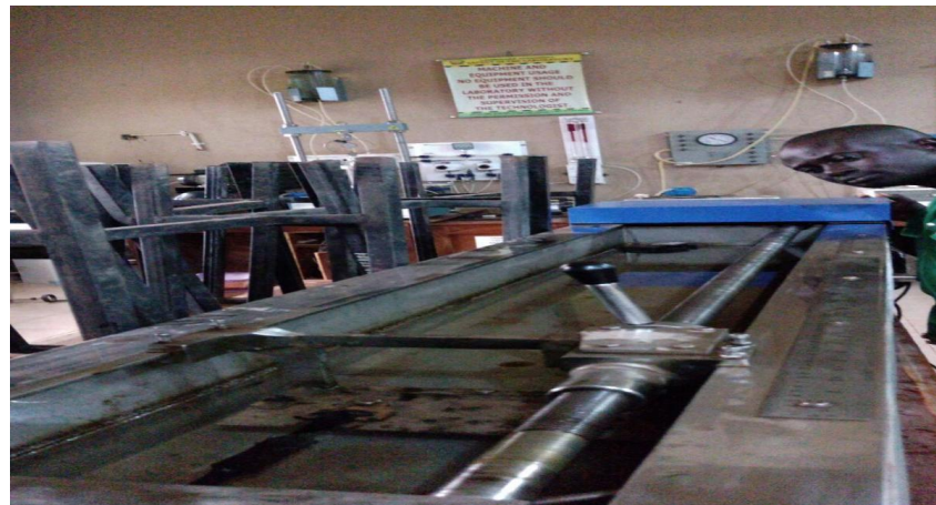
Figure 3: Ductility test Apparatus
