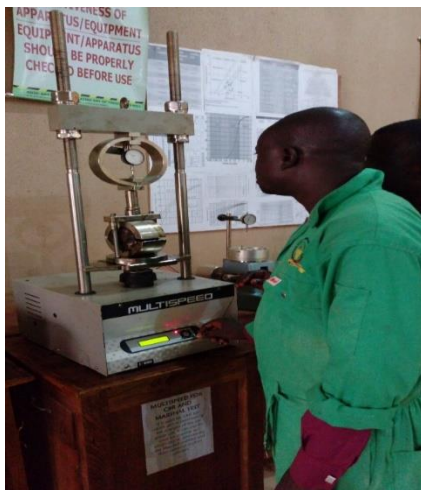
Figure 7b: Marshall Stability test set up
