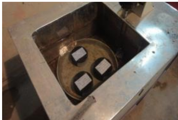
Figure 7a: Marshall Samples in Thermostatically Controlled Water Bath
