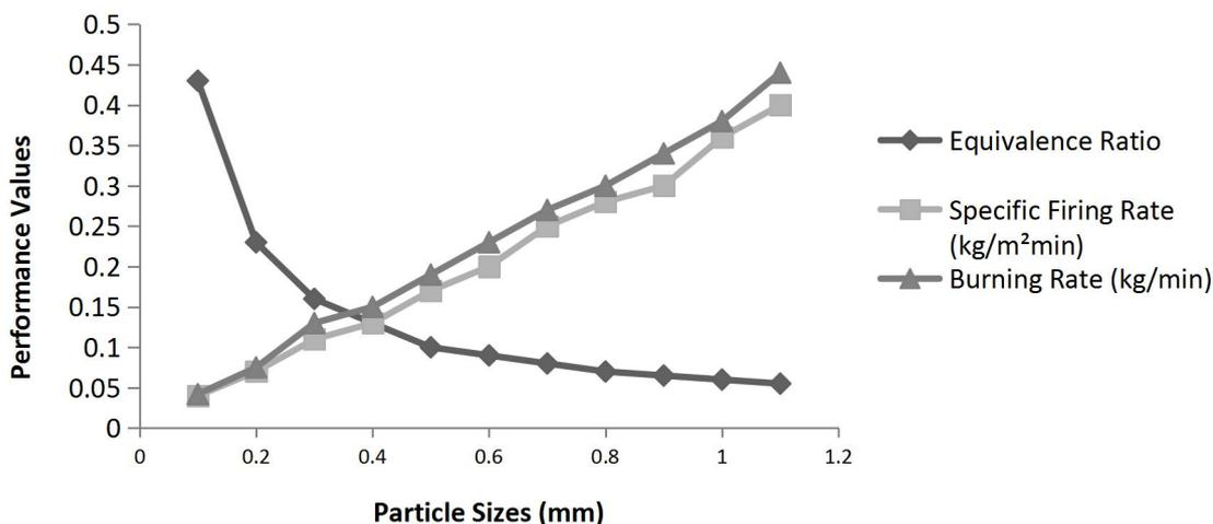
Figure 2: Effects of Maiganga Lignite Particle Sizes on Performance of the Combustor
