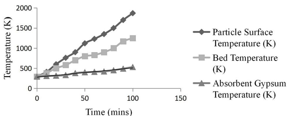
Figure 1: Maiganga Lignite Particle Surface, Bed and Gypsum Temperature against Time
