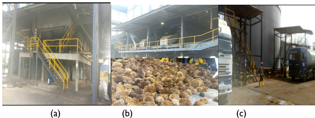
Figure 3. Functioning Facilities (a) Tilting Sterilizer (b) Stripper (c) SPO storage tank
