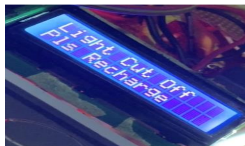
Figure 12: System under test with LCD displaying light cut off and recharge
