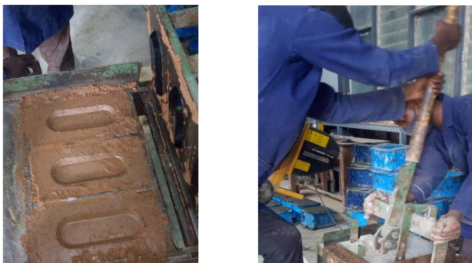
Figure 3: Pictorial presentation of the laterite block moulding work
