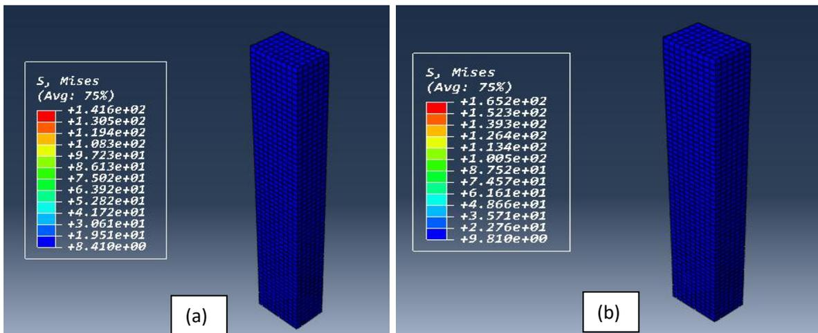
Figure 6 Von Mises Stress values under axial load (a) 1500 kN axial load (b) 1750 kN axial load
