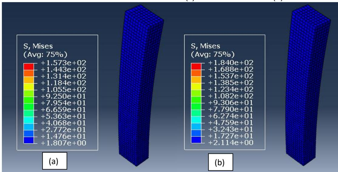
Figure 7. Von Mises Stress values on 25 mm-eccentric loading (a) 1500 kN (b) 1750 kN
