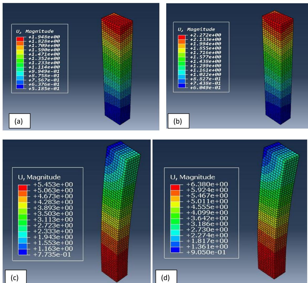
Figure 8. Deformation behaviour (a) 1500 kN, (b) 1750 kN, (c) 1500 kN @ Eccentricity of 25 mm (d) 1750 kN @ Eccentricity of 25 mm
