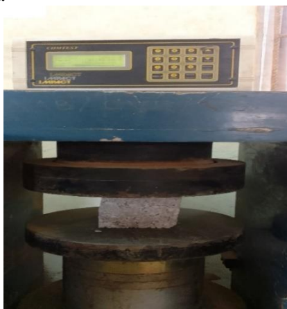
Figure 3: Compressive test on concrete sample.
