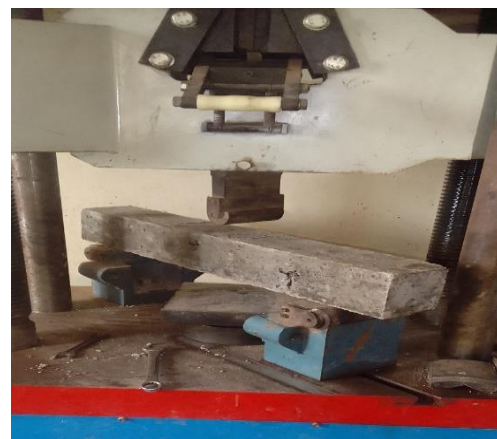
Figure 4: Three-point flexural strength test
