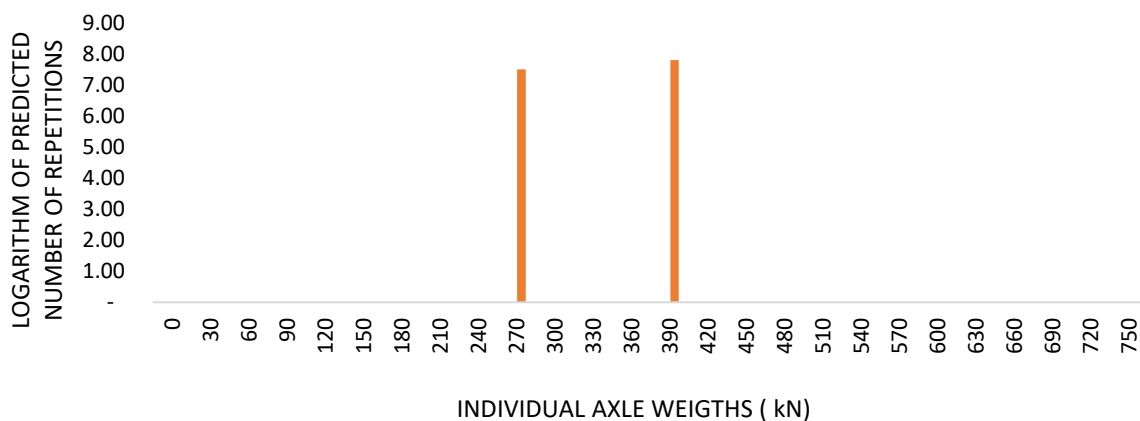
Figure 8: Predicted Number of Load Repetitions using GAF for Tridem Axle with Dual Tires Loads during 20year Design Period at Kaduna -Zaria Roadway
