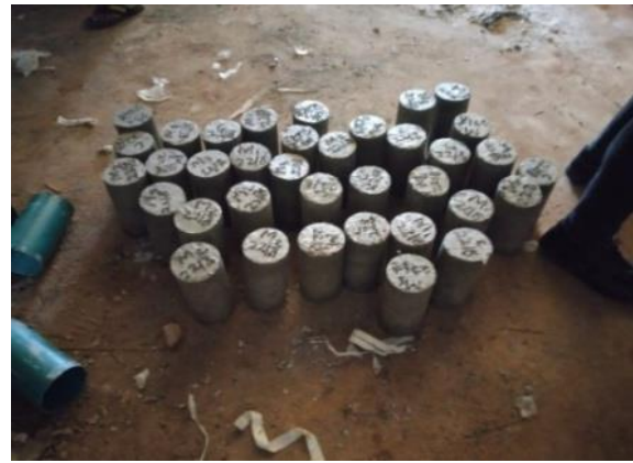
Figure 4: Pictorial view of the concrete for splitting tensile strength test
