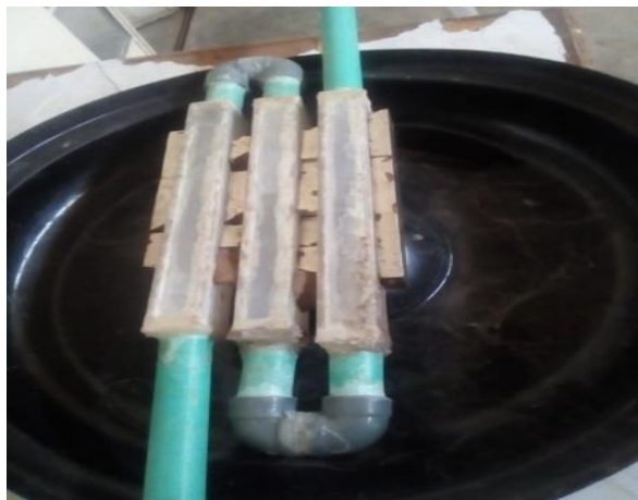
Figure 1: Magnetic water treatment unit with three pieces of magnets on both sides of the pipe
