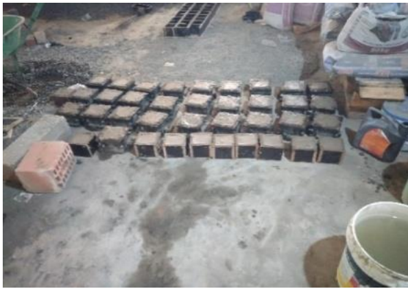
Figure 3: Pictorial view of the concrete for compressive strength test
